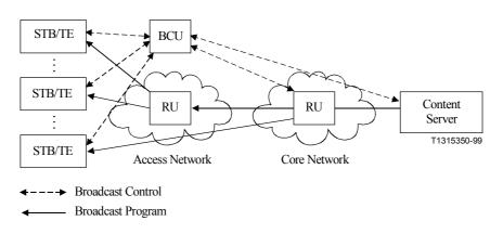
Figure 1/I.375.3 – Switched Digital Broadcast Service Architecture
