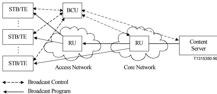
**Figure 1/I.375.3 – Switched Digital Broadcast Service Architecture**
