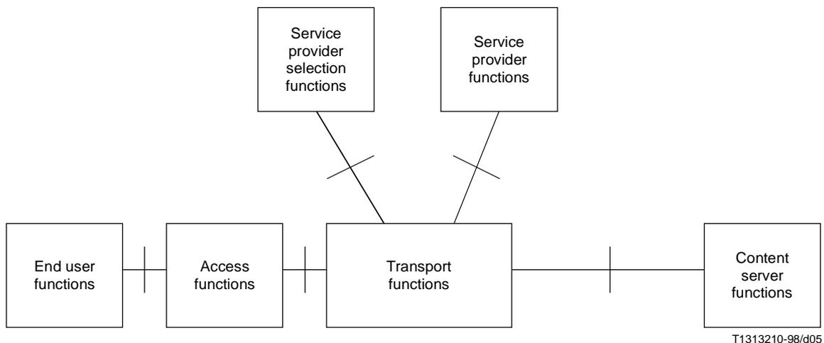
**Figure 5/I.375.1 – Reference configuration for multimedia retrieval services class**
