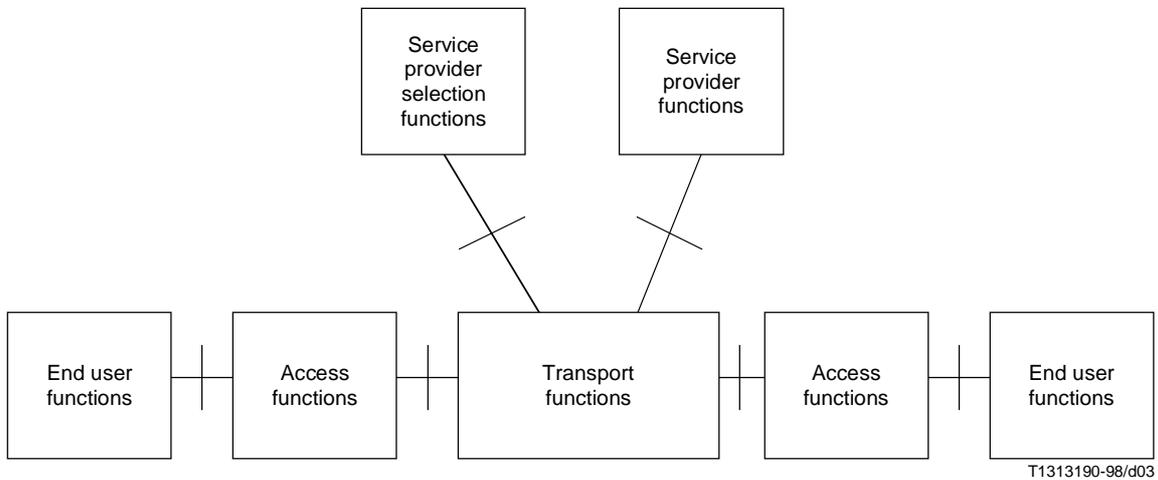
**Figure 3/I.375.1 – Reference configuration for multimedia conversation services class**
