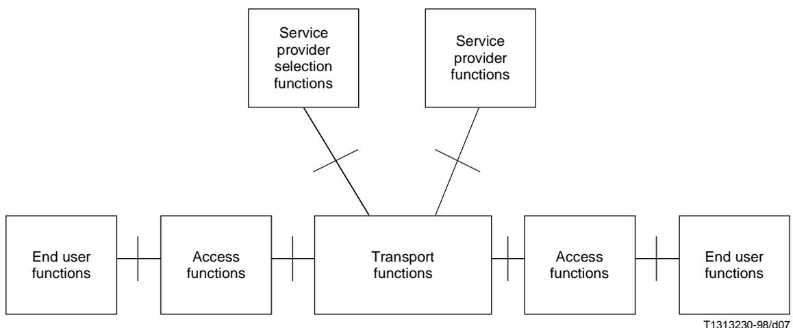
**Figure 7/I.375.1 – Reference configuration for multimedia message services class**
