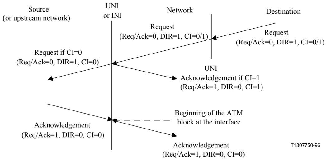
**Figure C.3/I.371 – BCR modification initiated by the destination**
