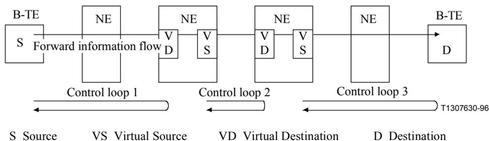
**Figure 15/I.371 – Example of a segmented virtual connection**
