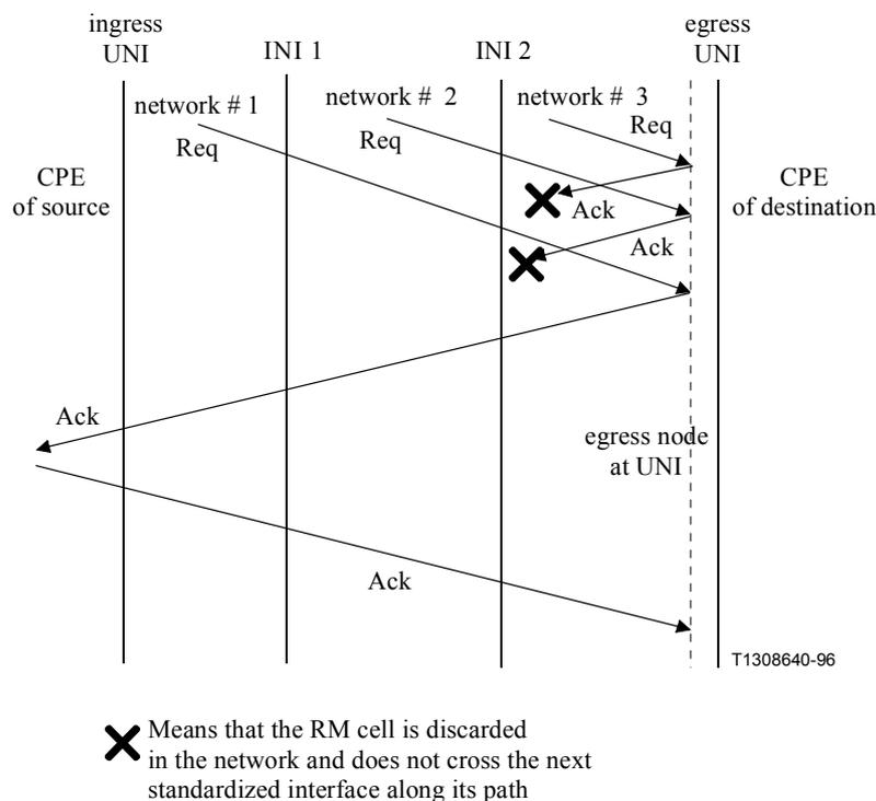
**Figure E.1/I.371 – BCR negotiations denial in the originating network, or a downstream network (RM cells have different sequence numbers)**
