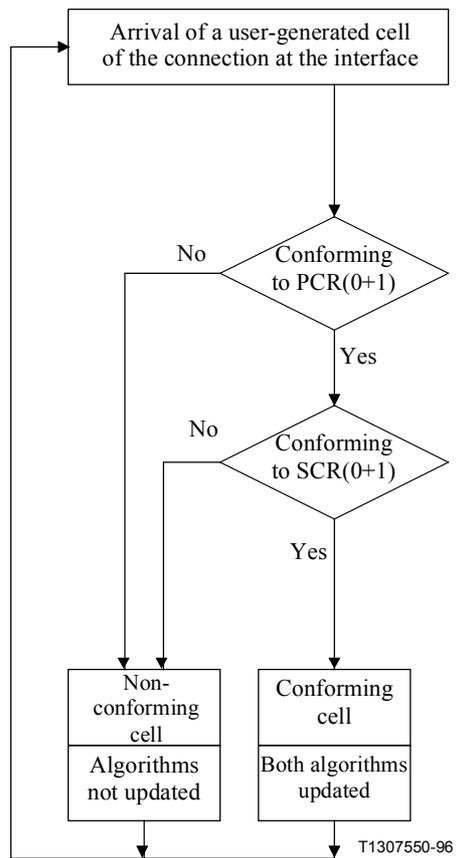
**Figure 7/I.371 – Conformance definition for SBR configuration 1**
