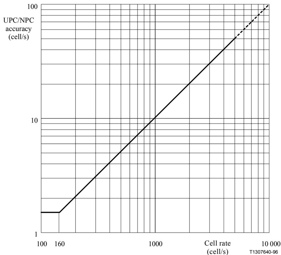
**Figure 17/L.371 – UPC/NPC accuracy requirement**
