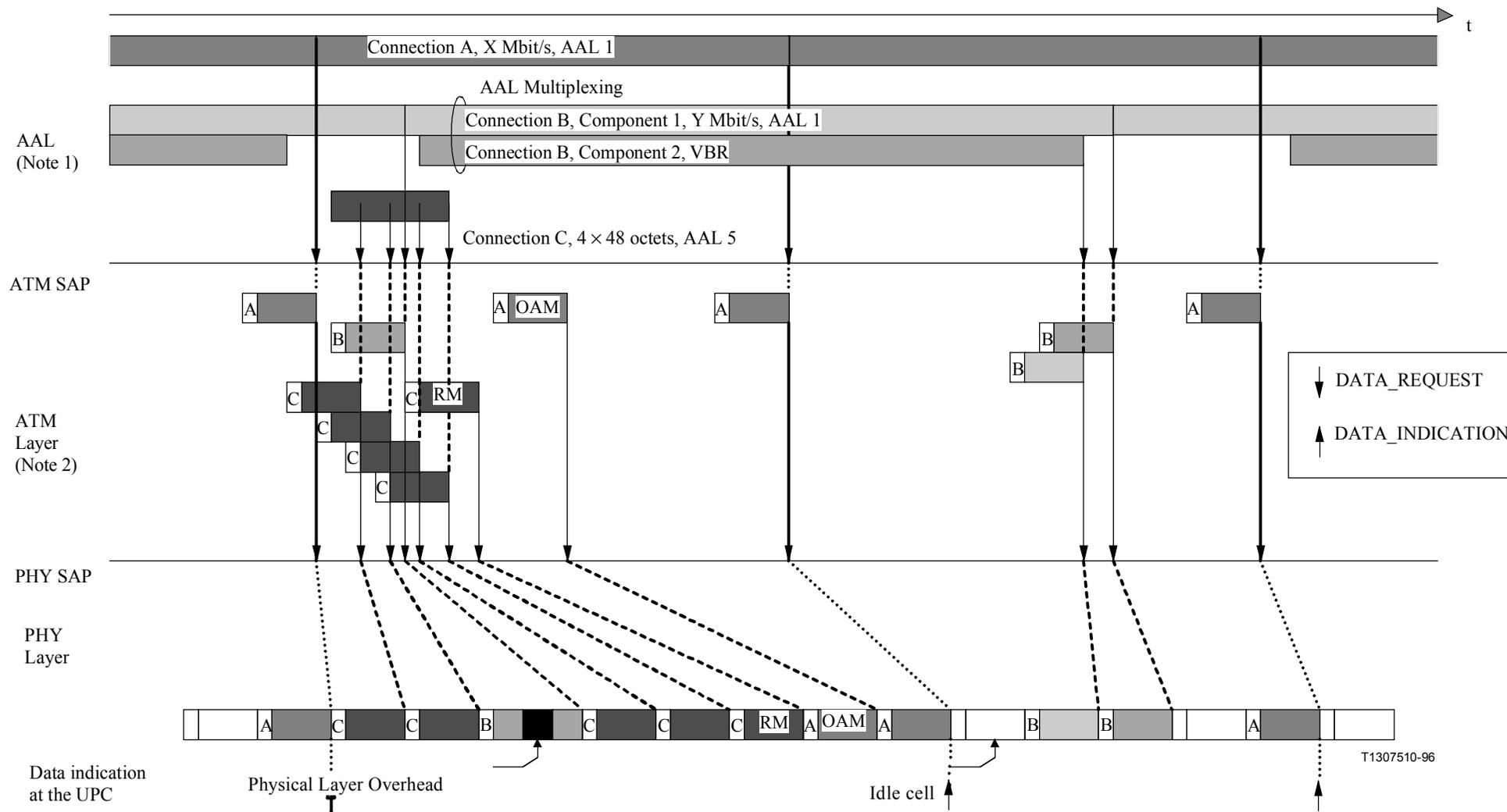
NOTE 1 – ATM SDUs are accumulated at the upper layer service bit rate. Besides, CDV may also originate in AAL multiplexing.
