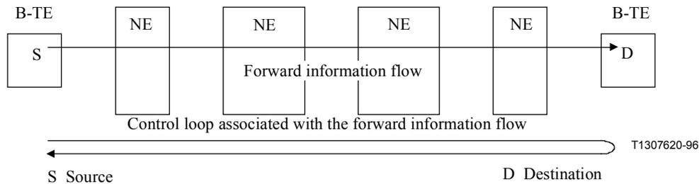
**Figure 14/I.371 – Example of a source to destination ABR control loop**
