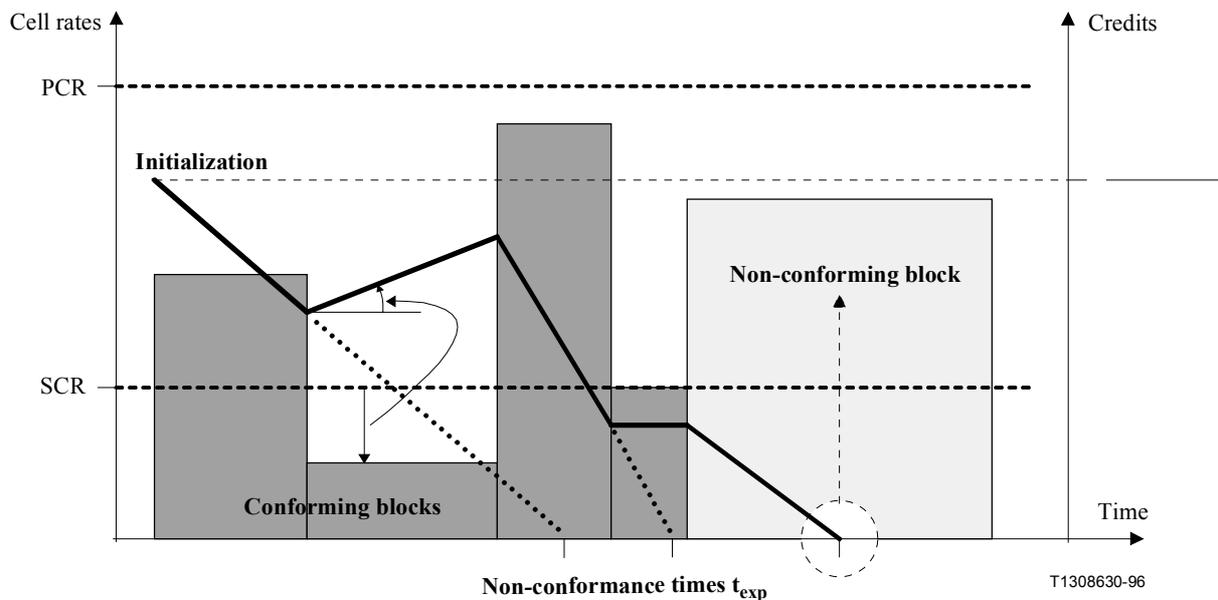
NOTE – This figure is for illustration purposes. The bold solid line represents the instantaneous number of credits. The slope of this curve is equal to the difference between the SCR and the BCR. Computation of  $t_{exp}$  for a given ATM block is based on the number of credits available at the ATM block boundary.
