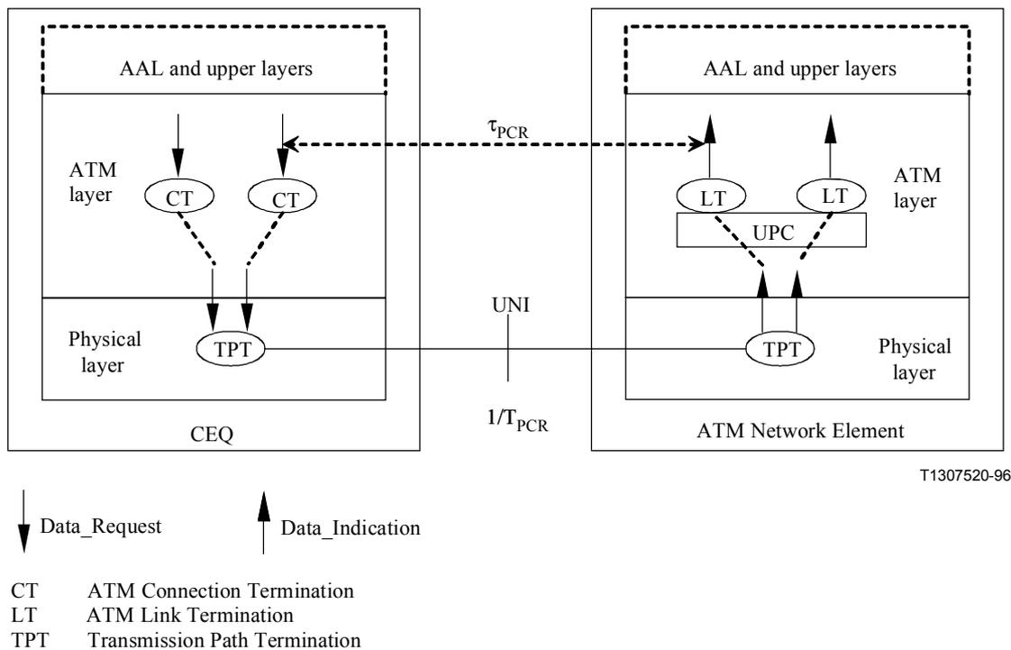
**Figure 4/I.371 – Reference configuration for the specification of traffic parameters**
