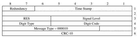
The format of dialled digit packets is shown in Figure K.1.
