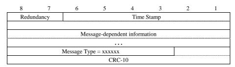
Figure 11-1/I.366.2 – Common facilities for type 3 packets
