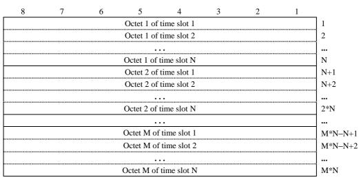
Figure J.1/I.366.2 – Circuit mode data packet format
