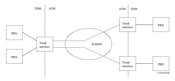
Figure 6-2/I.366.2 – Example deployment of narrow-band trunking
