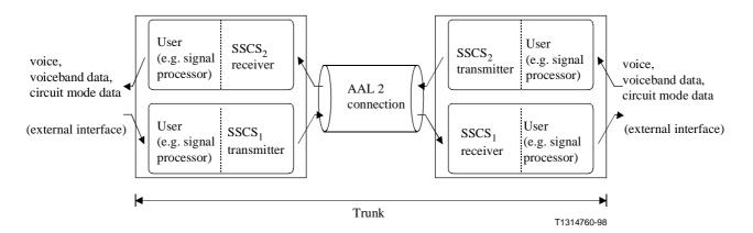
Figure 6-1/I.366.2 – Reference model of the SSCS for narrow-band trunking
