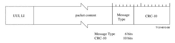
Figure 10-2/I.366.2 – Packet format type 3 – Fully protected
