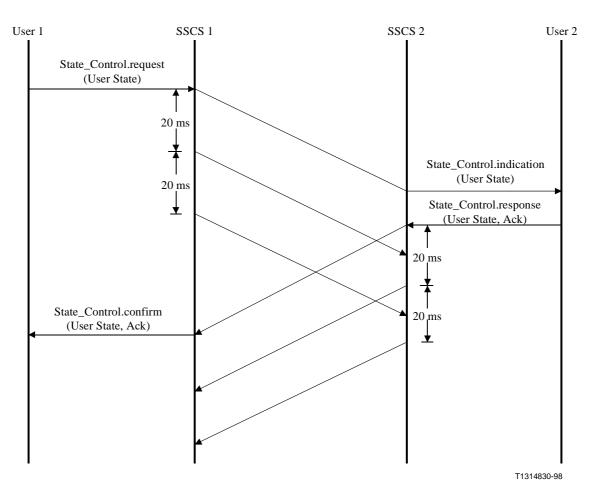
Figure O.2/I.366.2 – User state control message flow
