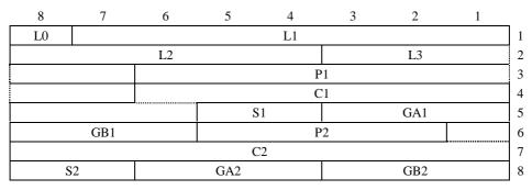
Figure H.3/I.366.2 – G.729-6.4 encoding data unit format
