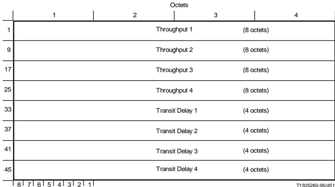
NOTE – Throughput *x* fields are binary counts in units of 100 bytes/sec. Transit Delay *x* fields are binary counts in units of milliseconds.
