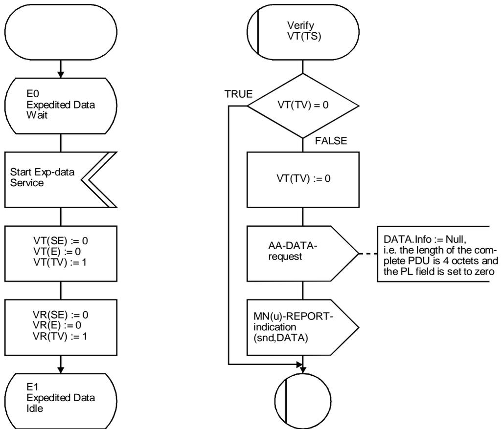
NOTE – The macro “Verify VT(TS)” is defined also in Figure D.3 (sheet 1 of 5); these two macros are identical and need to be present only once.
