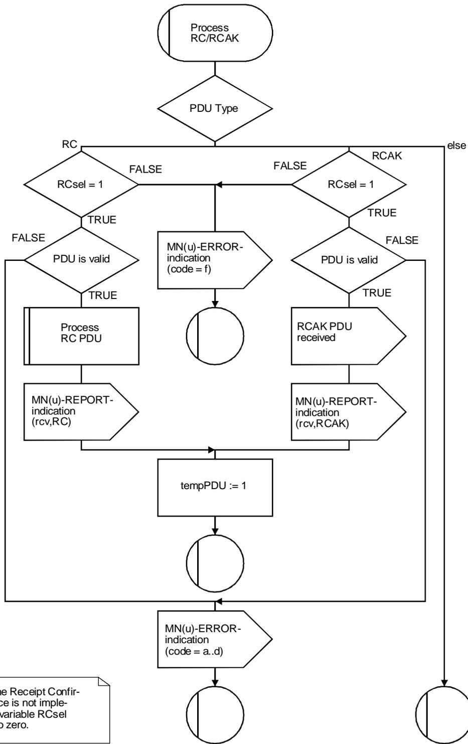
NOTE – If the Receipt Confirmation service is not implemented, the variable RCsel is clamped to zero.
