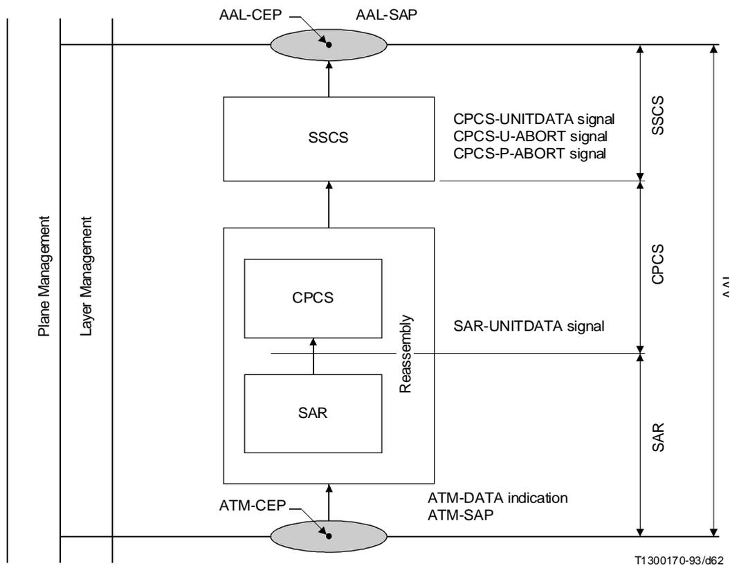
NOTE – Concerning the SSCS, the functional model is an example only. Possible functions in the SSCS (i.e. multiplexing) are not shown. The SSCS is specified in other Recommendations.
