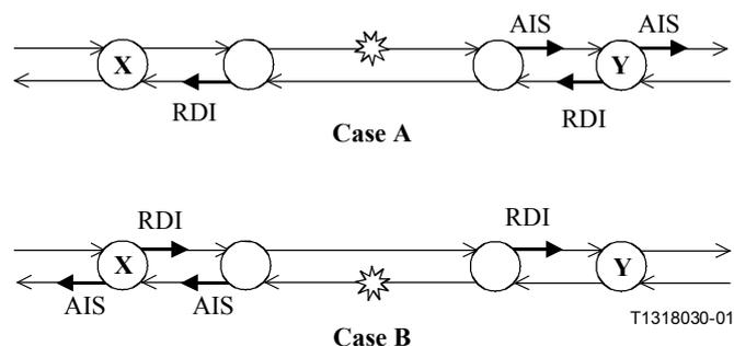
**Figure A.1/I.357 – A bidirectional connection delimited by MP X and Y**
