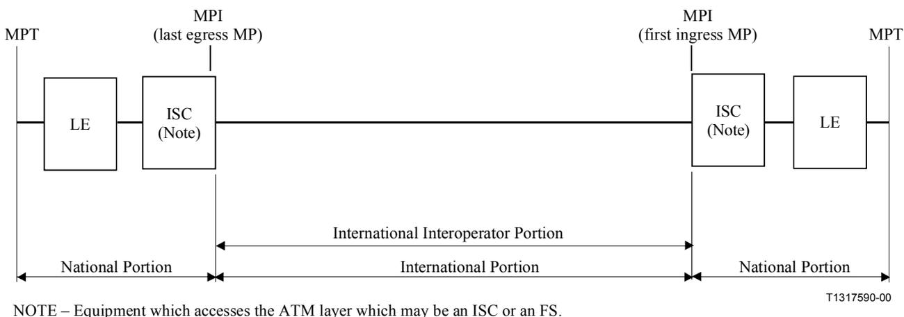
**Figure 2/I.357 – Connection with no international transit operators**
