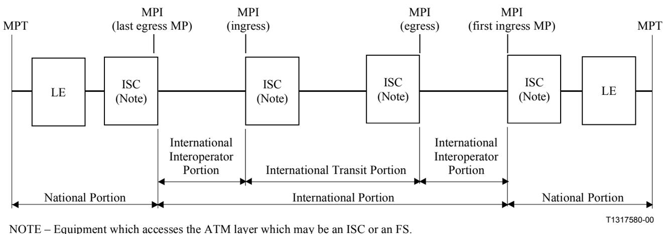
**Figure 1/I.357 – Connection with one international transit operator**
