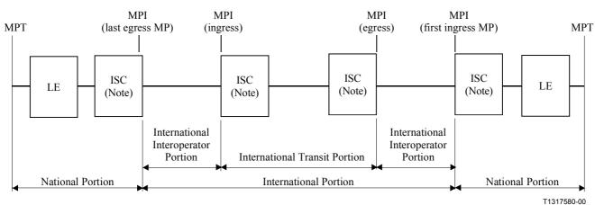
NOTE - Equipment which accesses the ATM layer which may be an ISC or an FS.
