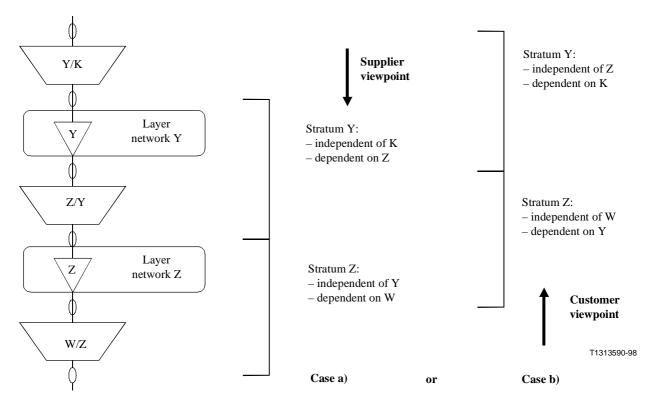
Figure 8/I.322 – The two cases of stratification
