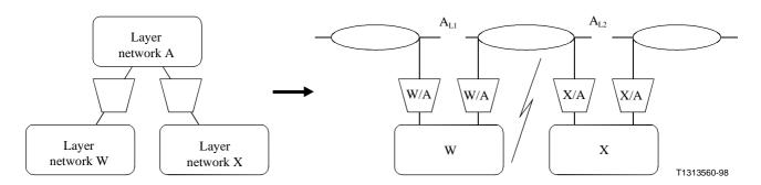
Figure 5/I.322 – Many-to-many relationships in partitioning a layer network
