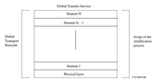
Figure 6/I.322 - Stratification process - General view
