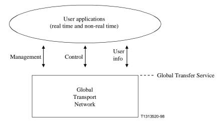
Figure 1/I.322 – The relationship between the users' applications and the global transport network
