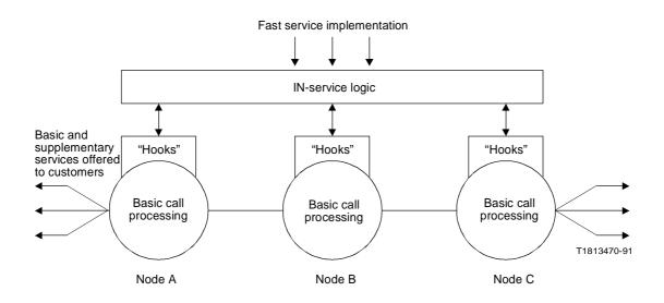
FIGURE 16 IN service processing model
