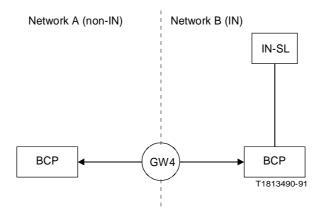
FIGURE 18 Gateway function between IN and non-IN
