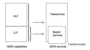
FIGURE 2/I.310 Relationship between telecommunication services and network capabilities
