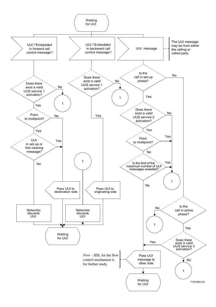
FIGURE 1/I.257.1 (sheet 2 of 3) User-to-User Signalling
