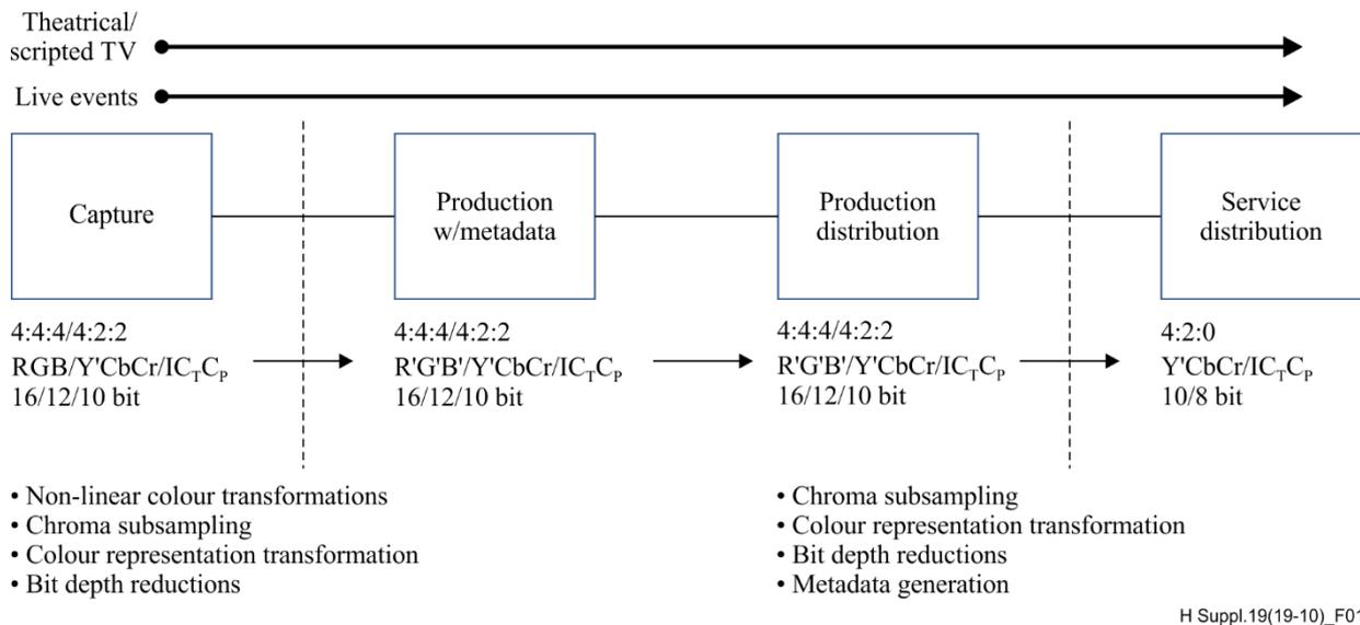
**Figure 1 – Video workflows through different carriage domains**
