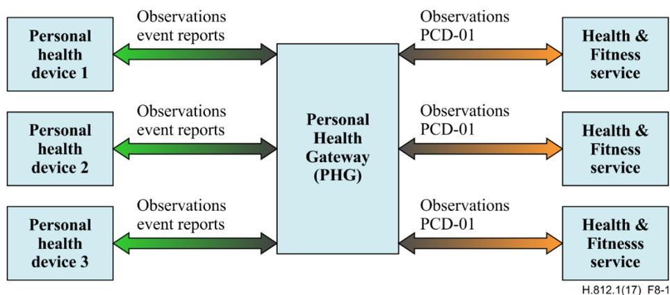
**Figure 8-1 – PHG block diagram**
