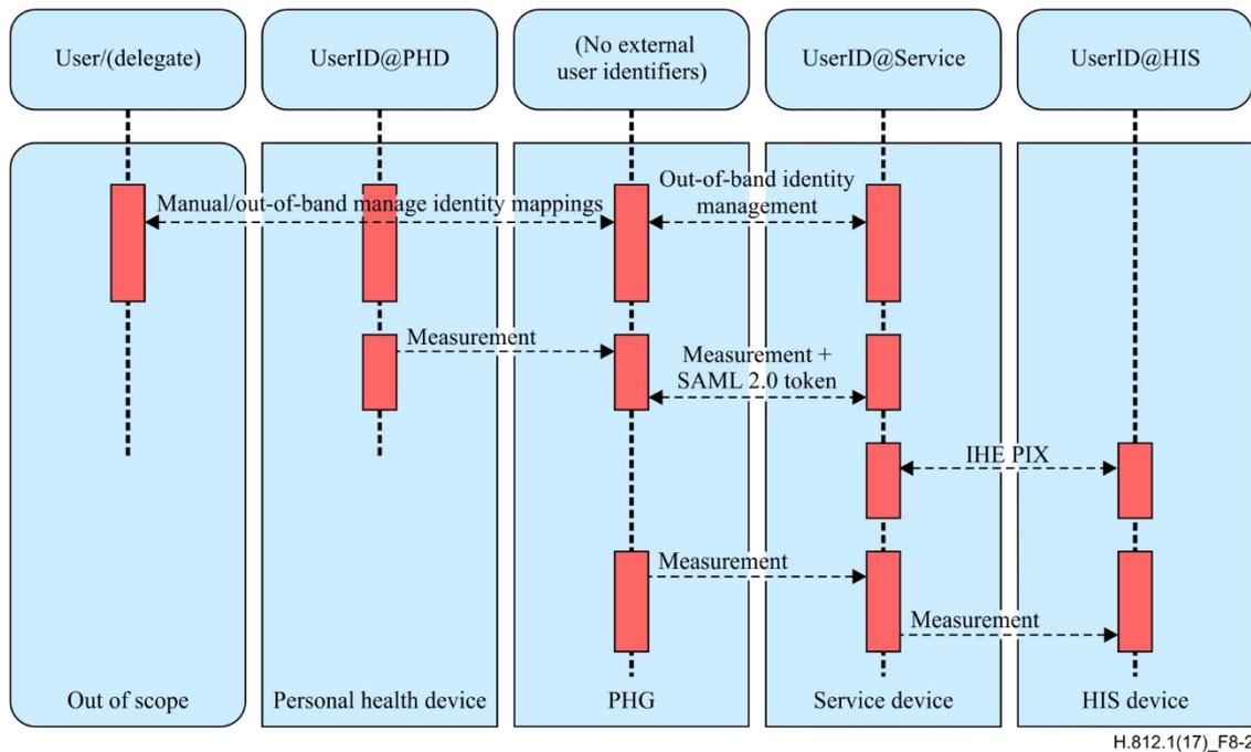
**Figure 8-2 – Identification and identity cross-referencing interactions**
