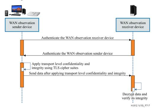
Figure 7-7 – Secure point-to-point communication sequence
