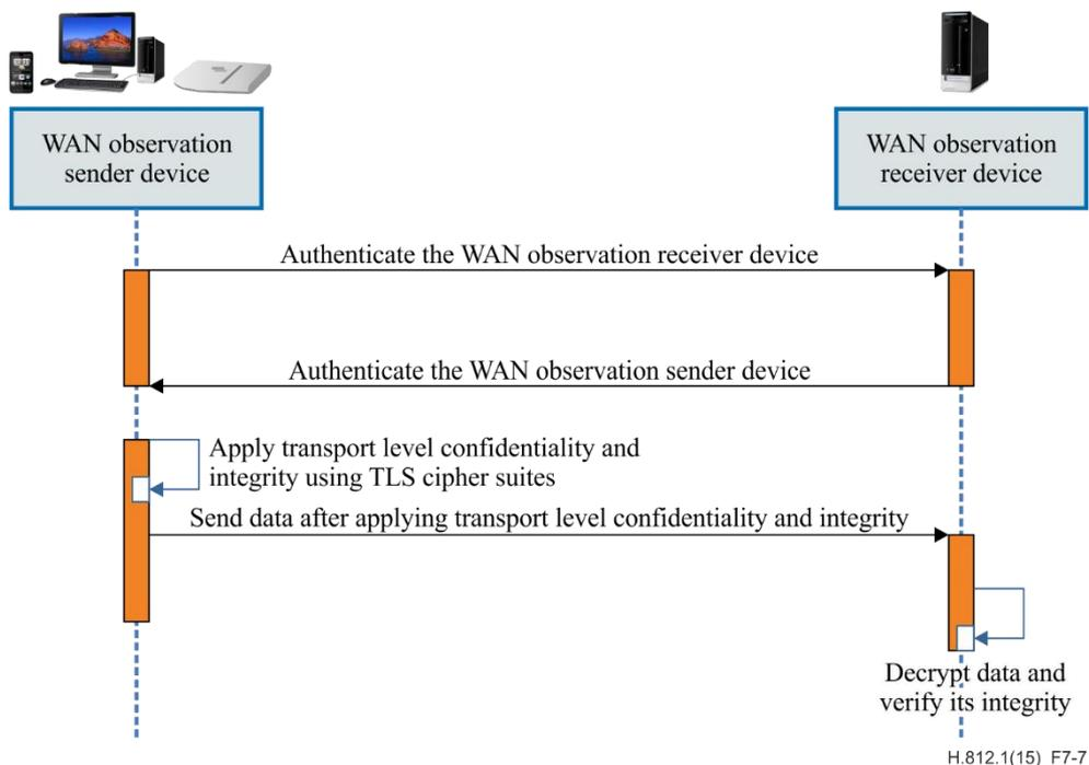
**Figure 7-7 – Secure point-to-point communication sequence**
