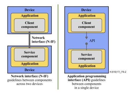
Figure 6-2 – Interfaces between components
