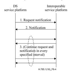
Figure 8-4 – Data flow of PULL type in IF-B
