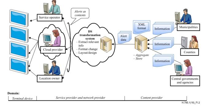
Figure I.2 – A cloud service provides only contents transformation
