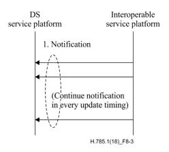
Figure 8-3 – Data flow of PUSH type in IF-B
