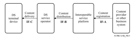
Figure 8-1 – Interfaces between each entity in the reference model
