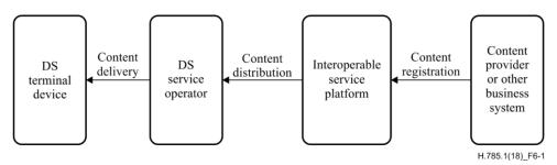
Figure 6-1 – Domain model with interoperable service platform
