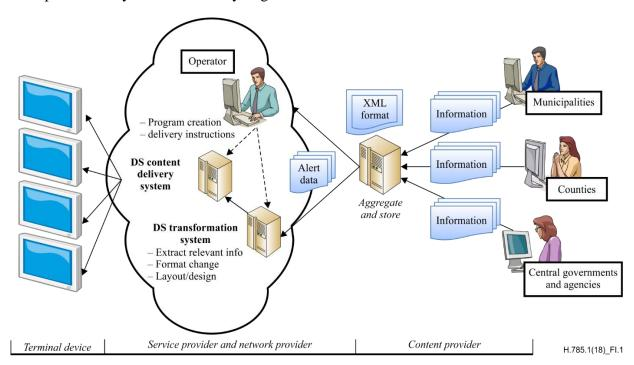
Figure I.1 – A cloud service provides both contents transformation and delivery
