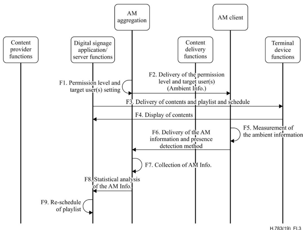
**Figure I.3 – Generic flow for the audience measurement based on ambient information**
