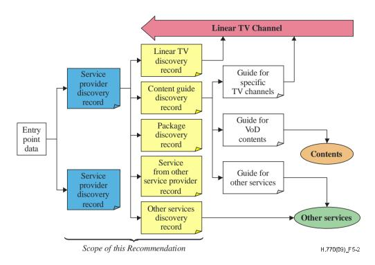
Figure 5-2 – From entry point data to service/content acquisition
