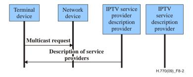
Figure 8-2 – Multicast request to receive the description of the available IPTV service providers
