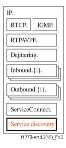
Figure V.2 – TR-135 Extension of FrontEnd.IP object structure
