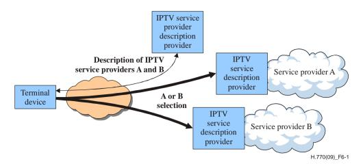
Figure 6-1 – Service provider discovery with a central IPTV service provider description provider
