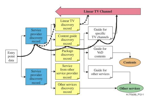
Figure 12-1 – Example of live channel selection through a service guide
