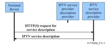
Figure 11-1 – HTTP or HTTP over TLS request for description of the IPTV services offered by a service provider
