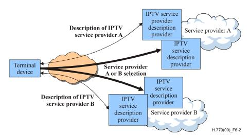
Figure 6-2 – Service provider discovery without a central service provider description provider
