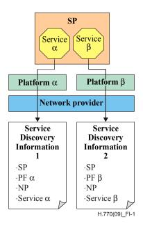
Figure I.1 – The case of providing different services from one service provider
