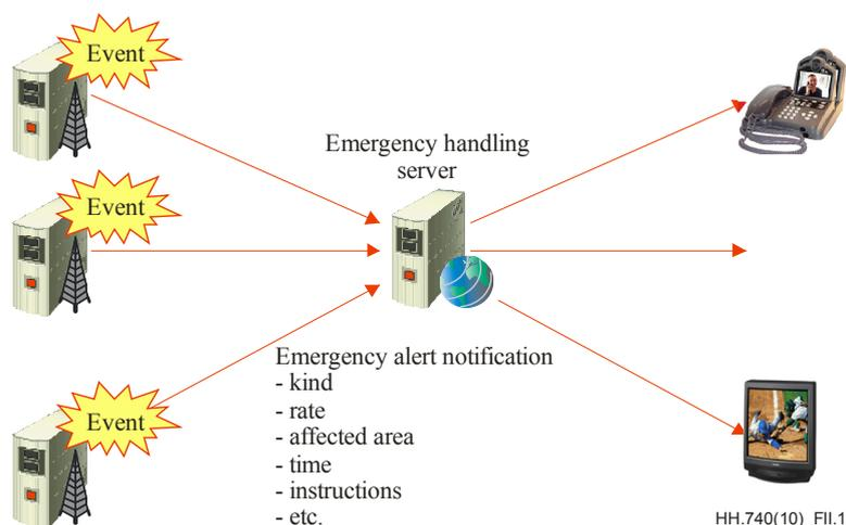
Figure II.1 – Application event notification scenario for emergency alert
