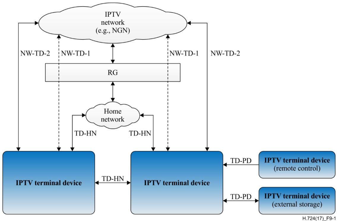
**Figure 9-1 – Physical interfaces that support interworking among multiple IPTV terminal devices**
