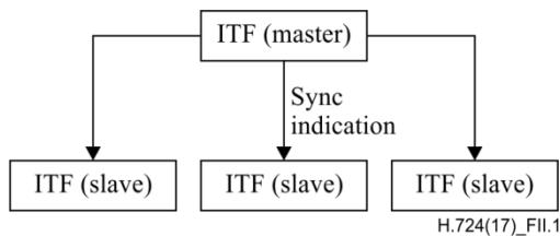
**Figure II.1 – Master-slave synchronization schema**
