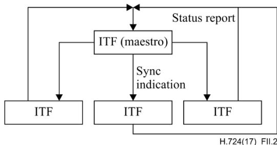
**Figure II.2 – Maestro synchronization schema**
