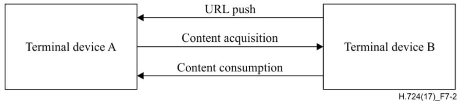
**Figure 7-2 – Interworking between two terminal devices (URL push mode)**
