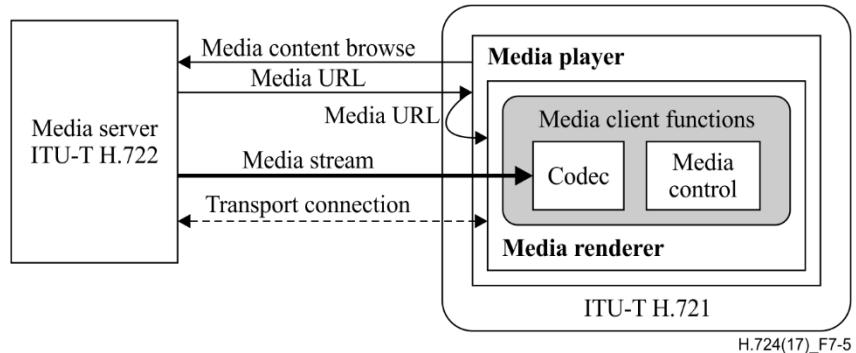
**Figure 7-5 – Interworking model for ITU-T H.721 terminal device**
