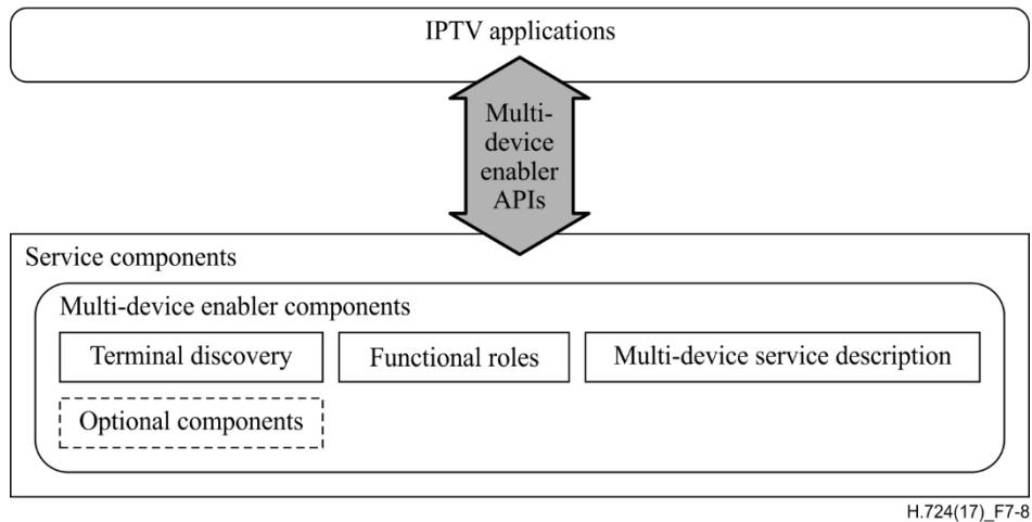
**Figure 7-8 – Multi-device enabler APIs**
