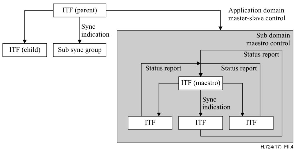
**Figure II.4 – An instance of a hierarchical distribution synchronization schema**
