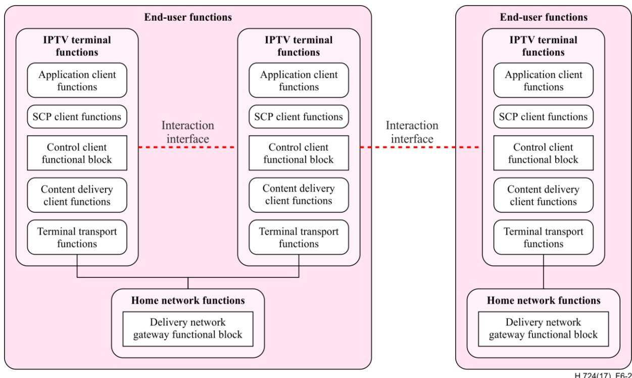
**Figure 6-2 – High-level overview of interworking between terminal devices**
