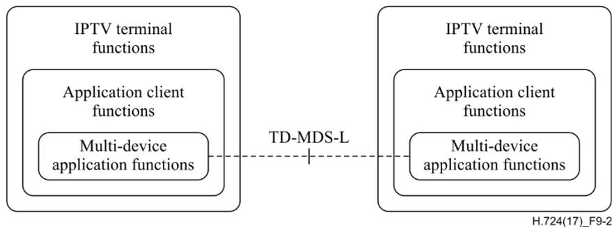
**Figure 9-2 – Logical interface between multi-device application functions**
