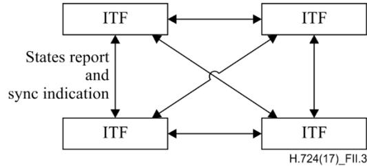
**Figure II.3 – Distributed synchronization schema**
