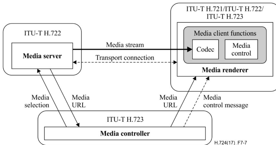
Figure 7-7 – Interworking model for an ITU-T H.723 terminal device
