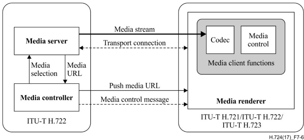
**Figure 7-6 – Interworking model for ITU-T H.722 terminal device**
