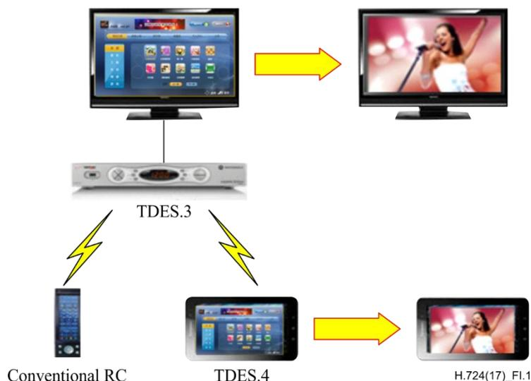
**Figure I.1 – EPG and media content sharing over multiple TDs**
