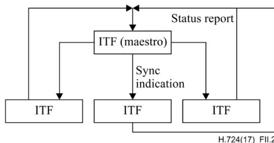
Figure II.2 – Maestro synchronization schema
