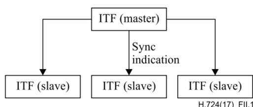
Figure II.1 – Master-slave synchronization schema
