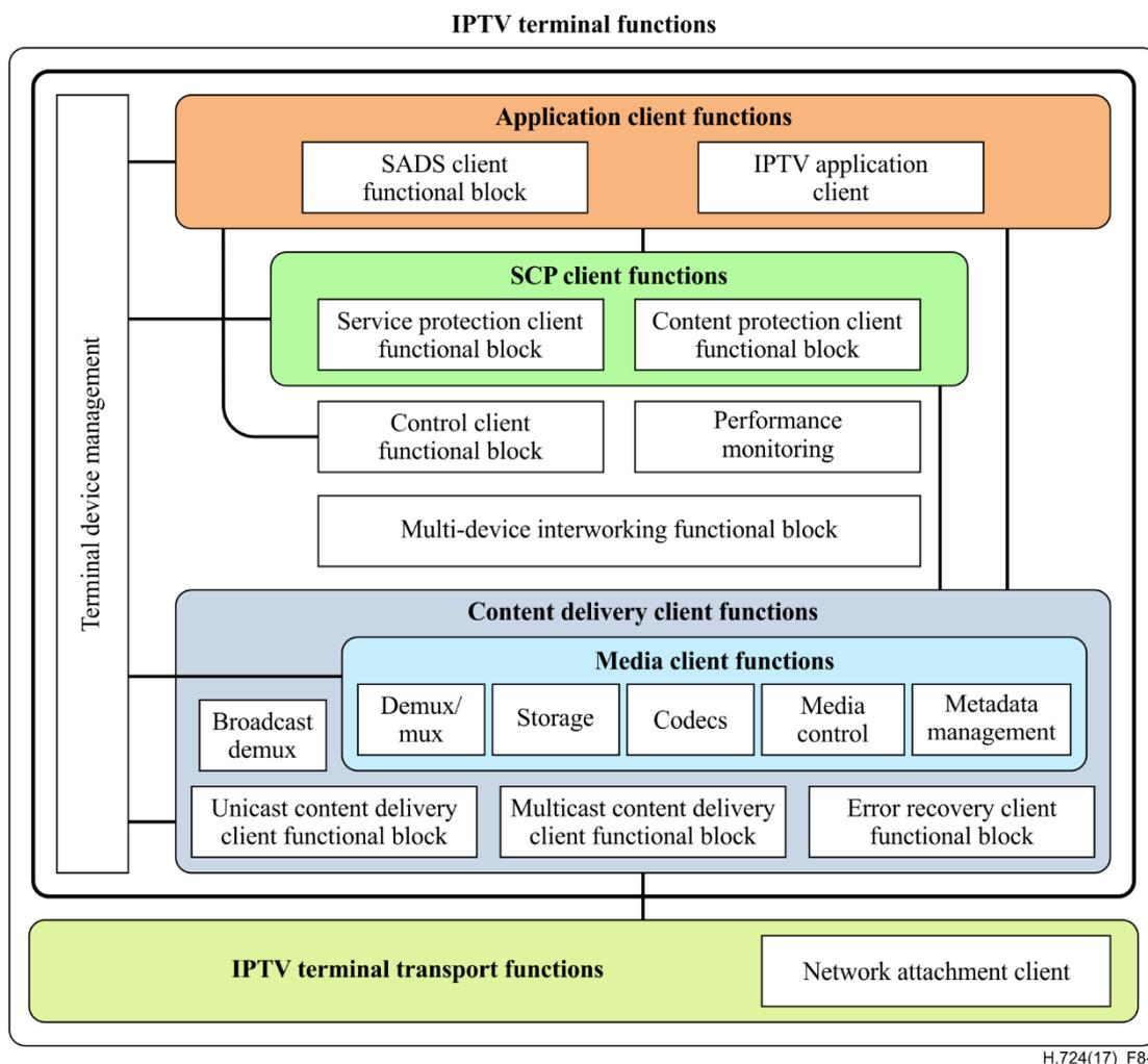
**Figure 8-1 – IPTV terminal functions including interworking based on [ITU-T H.720]**
