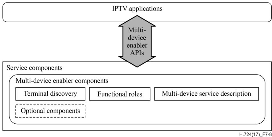
**Figure 7-8 – Multi-device enabler APIs**
