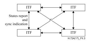
Figure II.3 – Distributed synchronization schema
