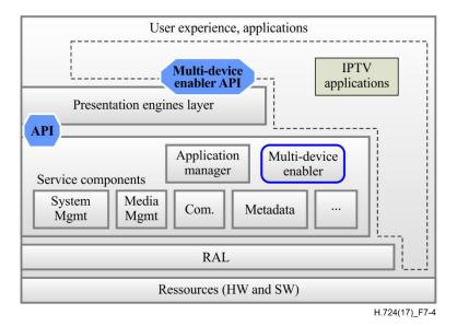
Figure 7-4 – Application framework to support multi-device service
