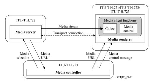
Figure 7-7 – Interworking model for an ITU-T H.723 terminal device
