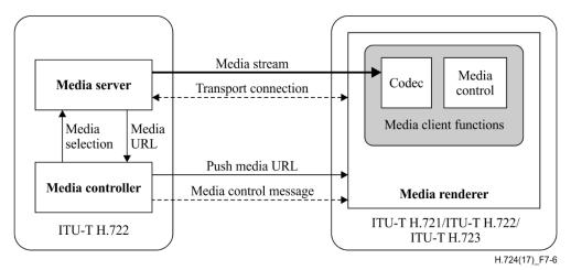
Figure 7-6 – Interworking model for ITU-T H.722 terminal device
