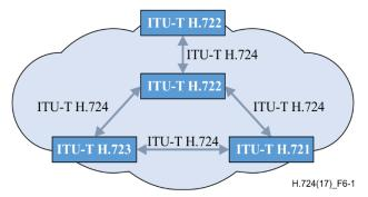
NOTE – Albeit basic model TDs [ITU-T H.721] and mobile model TDs, [ITU-T H.723] could interwork with the same model TD if they implement certain additional non-required features, this is not recommended (see Table 7-1). For this reason, self-interworking is represented in Figure 6-1 only for full-fledged TD models [ITU-T H.722].
