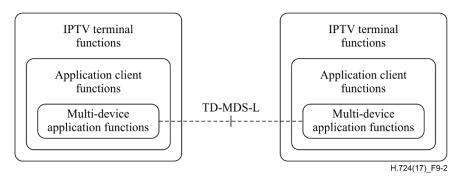
Figure 9-2 – Logical interface between multi-device application functions
