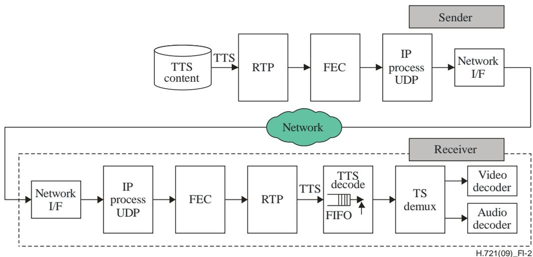
**Figure I.2 – System overview of timestamped TS clock synchronization**
