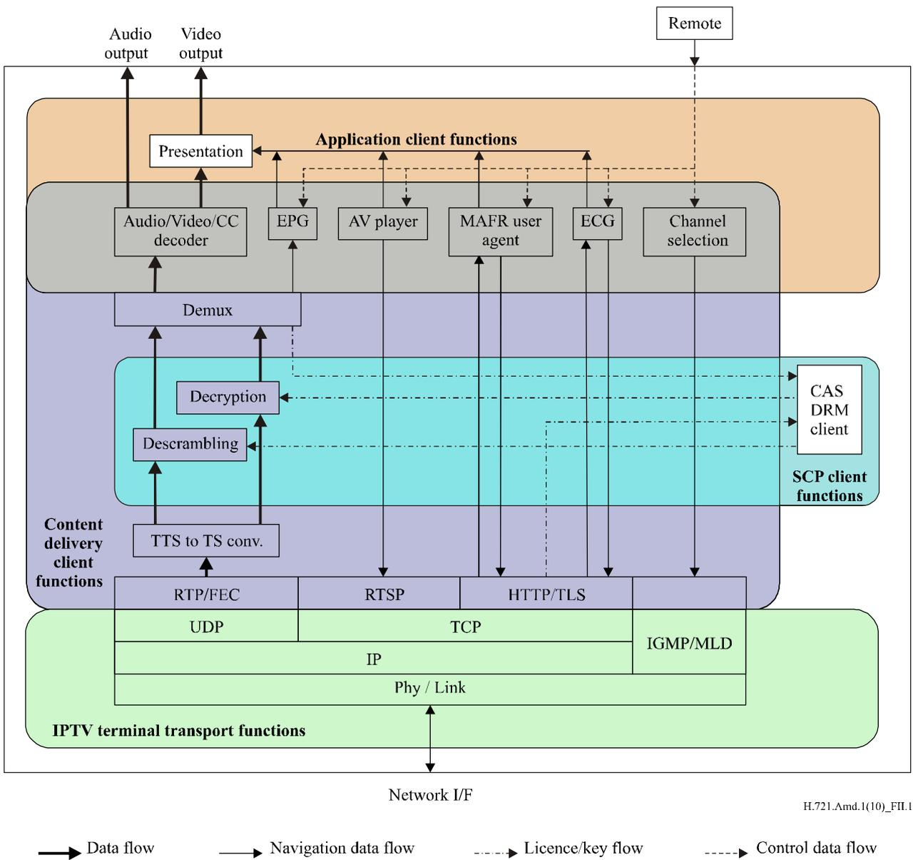
**Figure II.1 – Implementation example of the IPTV terminal functions**
