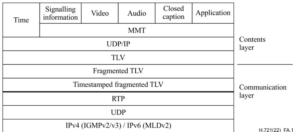
Figure A.1 – Protocol stack of MMT-based IPTV systems
