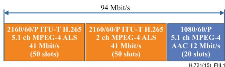
**Figure III.1 – Example configuration for two 4K with lossless streams and one HD stream with MPEG-4 AAC**
