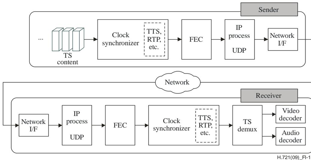
Figure I.1 – System overview of the clock synchronization
