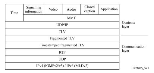
Figure A.1 – Protocol stack of MMT-based IPTV systems
