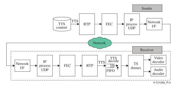
Figure I.2 – System overview of timestamped TS clock synchronization
