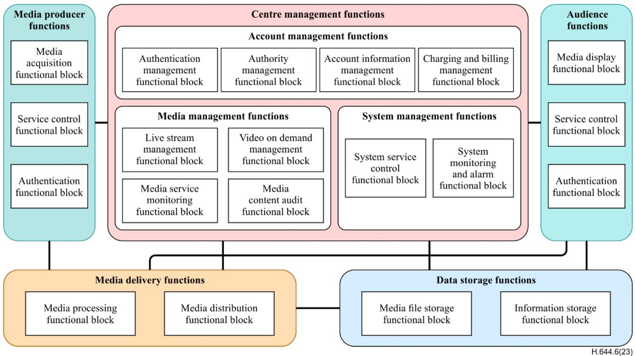
**Figure 6-1 – Functional architecture of video distribution system**
