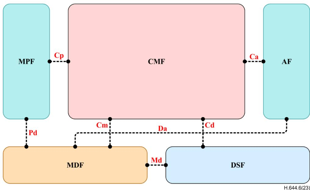
**Figure 8-1 – Reference points for VDS architecture**
