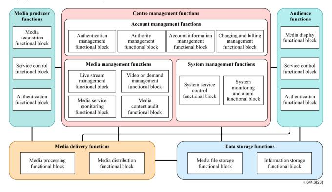
Figure 6-1 – Functional architecture of video distribution system
