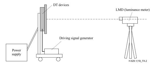
Figure A.2 – Example of equipment for measurement of greyscale luminance
