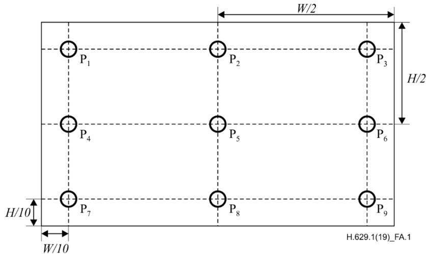
**Figure A.1 – Standard measurement positions are at the centres of all rectangles P<sub>1</sub>-P<sub>9</sub>**
