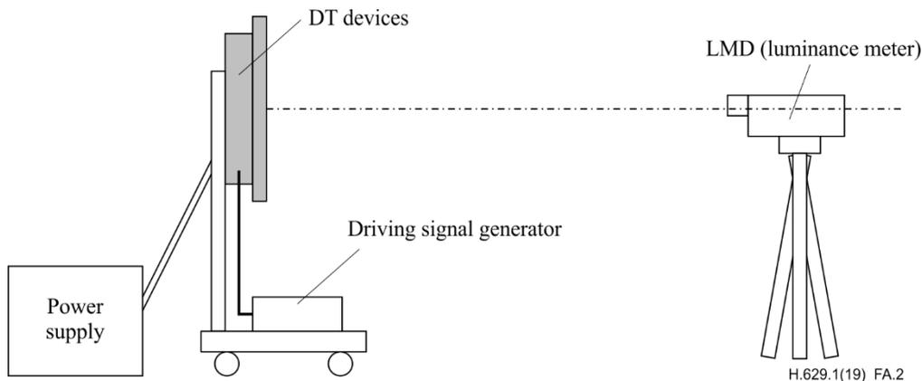
**Figure A.2 – Example of equipment for measurement of greyscale luminance**
