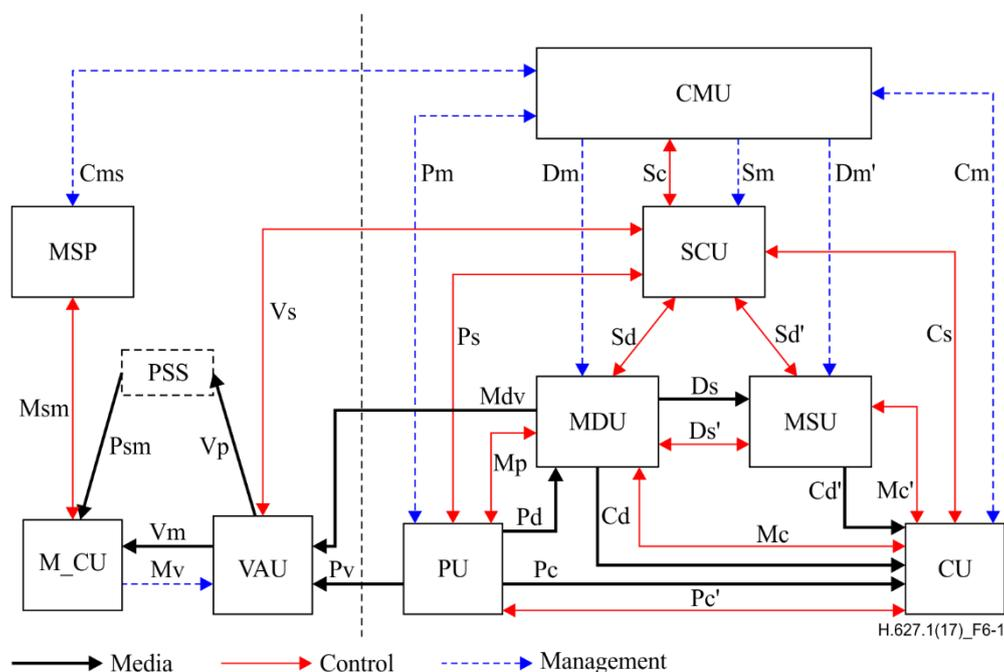
**Figure 6-1 – Functional architecture framework of mobile visual surveillance**
