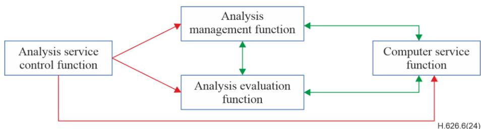
**Figure 6-3 – Function modules of VAEU**
