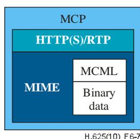
**Figure 6-7 – MCP structure**
