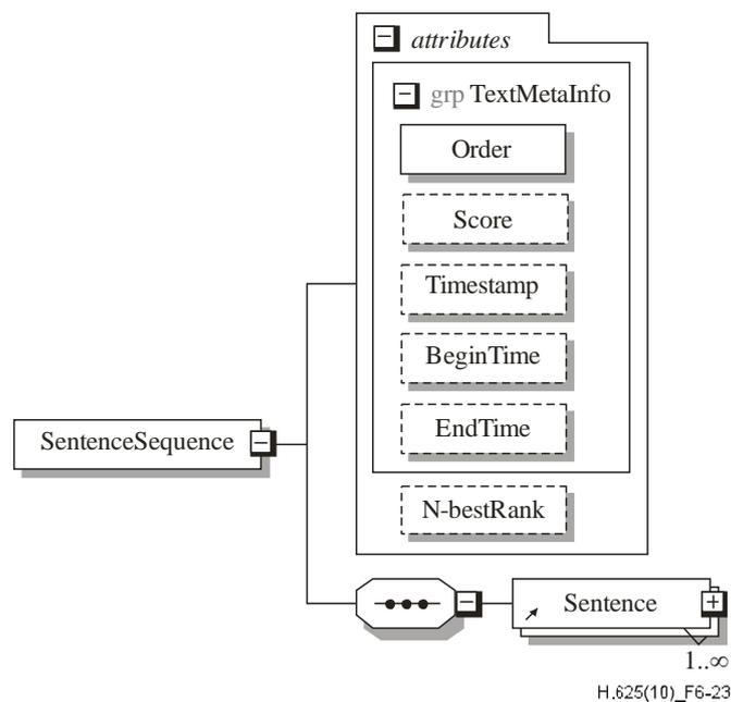
**Figure 6-23 – Structure of a "SentenceSequence" element**
