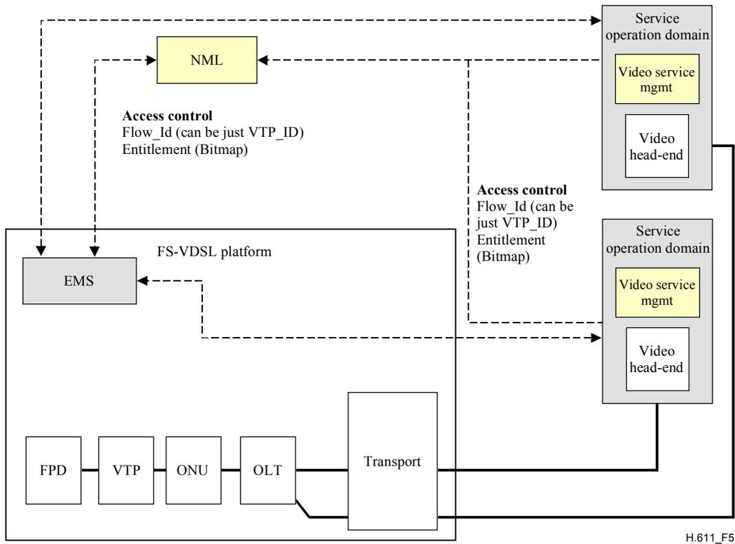
Figure 5/H.611 – Access control channels
