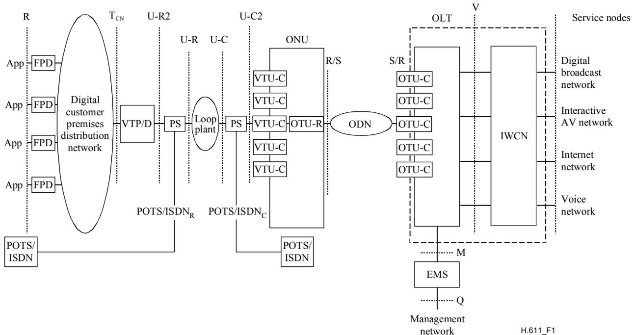
**Figure 1/H.611 – FS-VDSL reference model**
