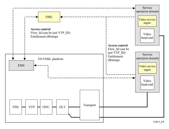
Figure 5/H.611 – Access control channels
