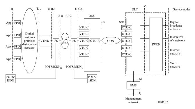
Figure 1/H.611 – FS-VDSL reference model
