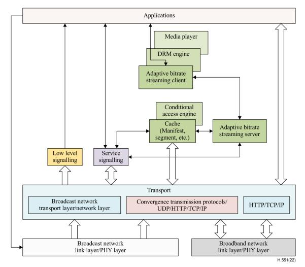
Figure 6 – Reference receiver model of in-vehicle devices
