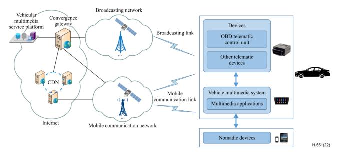
Figure 2 – A system diagram for VMS multimedia applications
