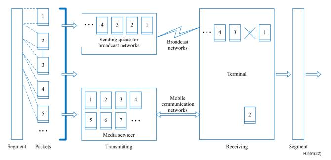
**Figure 4 – The processing of convergence transmission**
