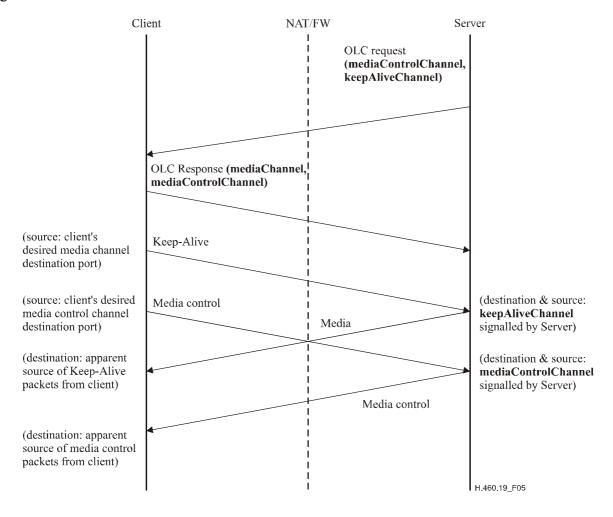
Figure 5/H.460.19 – Opening an LC toward the H.460.19 client
