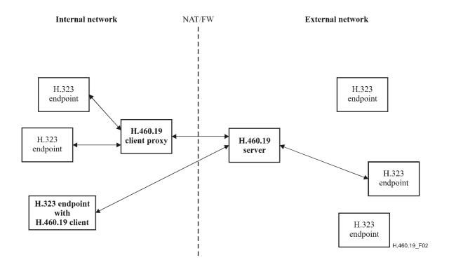
Figure 2/H.460.19 – Decoupled H.460.19 architecture
