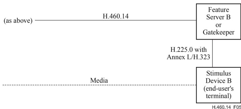
**Figure 5/H.460.14 – Stimulus signalling using Annex L/H.323**
