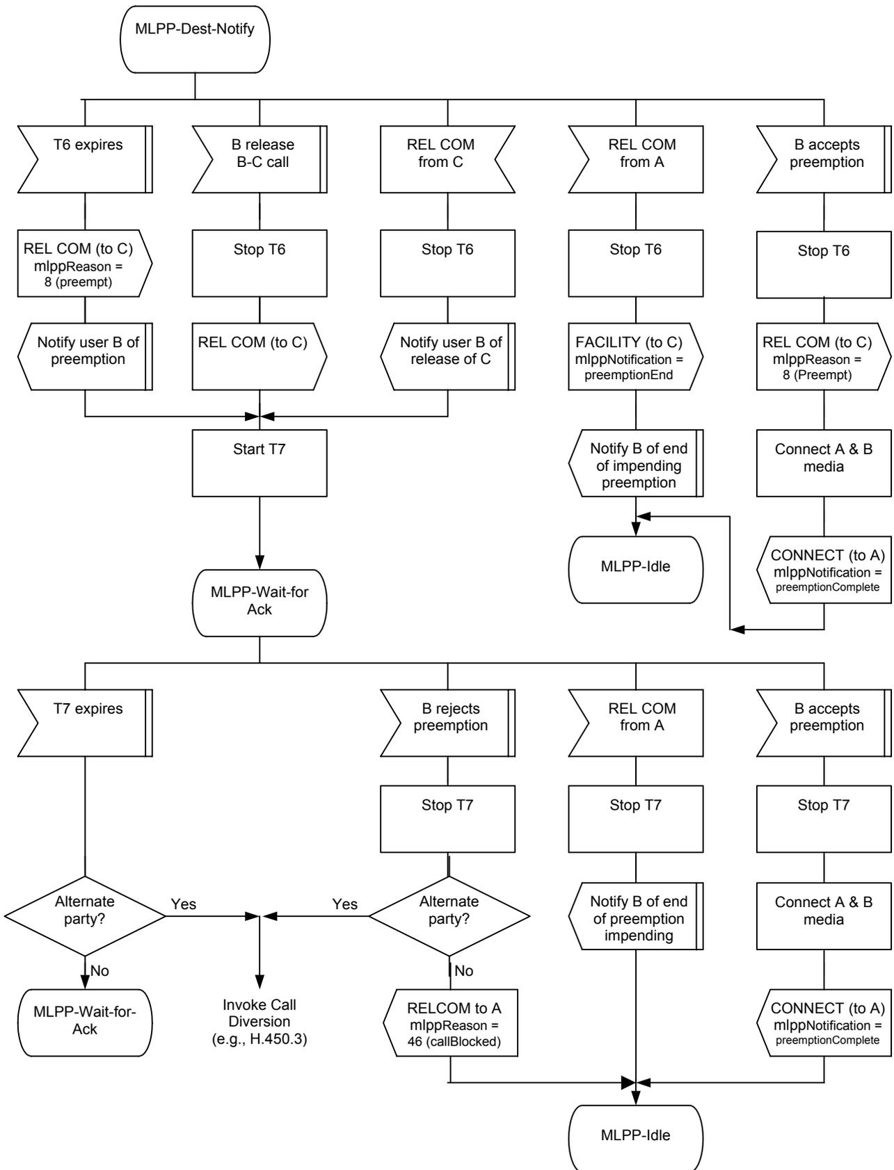
Figure 15/H.460.14 – Endpoint B SSDL (sheet 2 of 2)
