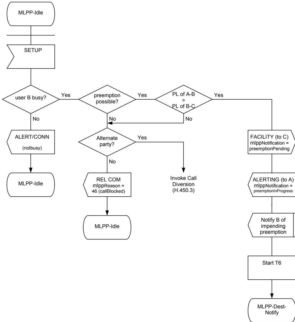
Figure 14/H.460.14 – Endpoint B SDL (sheet 1 of 2)
