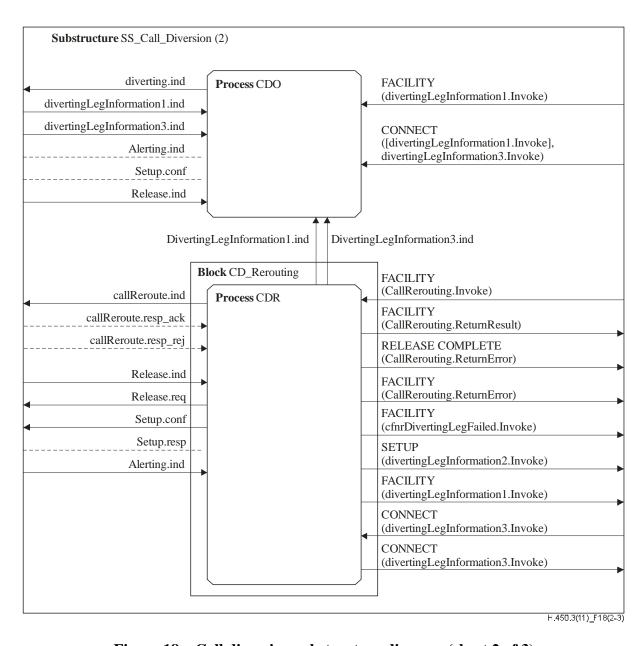
Figure 18 – Call diversion substructure diagram (sheet 2 of 3)
