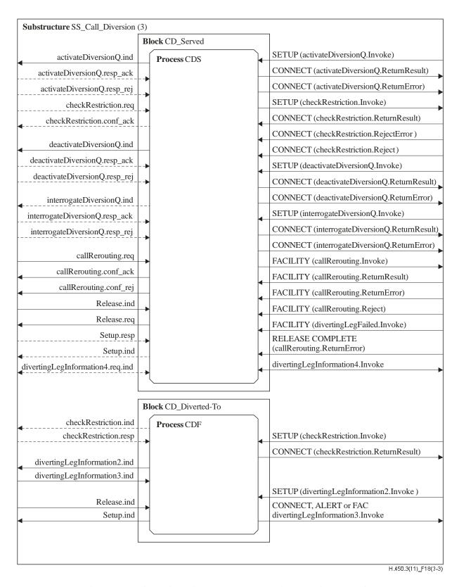
Figure 18 – Call diversion substructure diagram (sheet 3 of 3)
