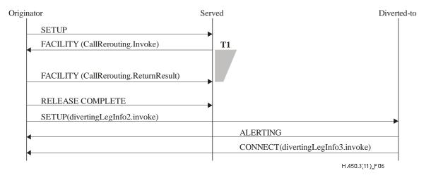
Figure 6 – Signalling flow for call forwarding immediate (CFU, CFB) with rerouting
