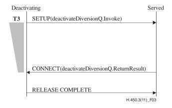
Figure 3 – Signalling flow for remote deactivation of call forwarding
