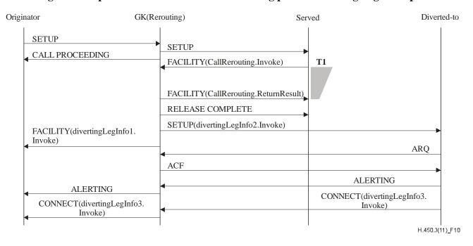
Figure 10 – Signalling flow for call forwarding partial rerouting in gatekeeper
