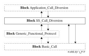
Figure 17 – Call diversion block diagram
