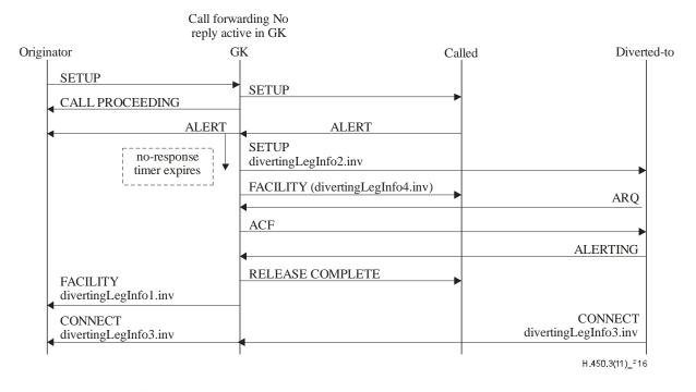
Figure 16 – Signalling flow for CFNR invoked by gatekeeper on user B no answer
