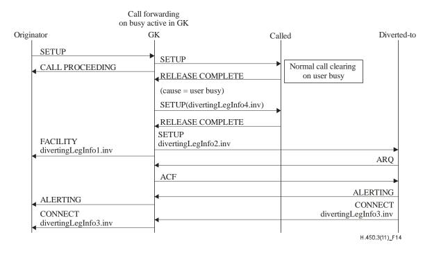
Figure 14 - Signalling flow for CFB invoked by gatekeeper on user B busy
