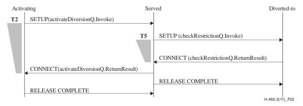
Figure 2 – Signalling flow for remote activation of call forwarding
