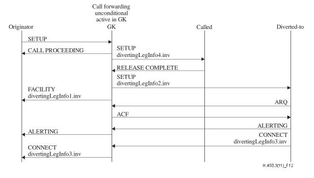
Figure 12 - Signalling flow for CFU invoked by gatekeeper
