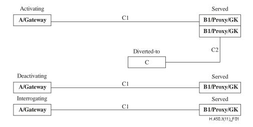
Figure 1 – Operational model for remote activation/deactivation/interrogation of call forwarding
