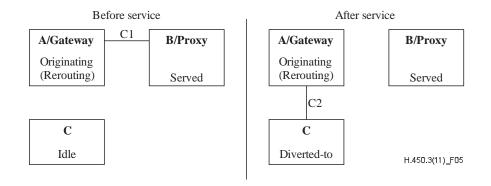
Figure 5 – Operational model for call forwarding immediate (CFU, CFB) with rerouting
