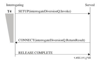
Figure 4 – Signalling flow for remote interrogation of call forwarding
