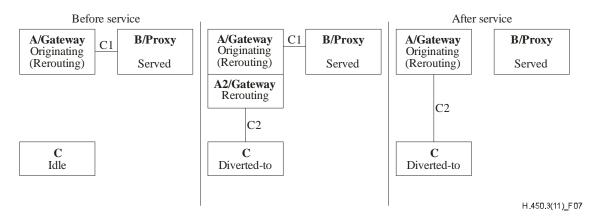
Figure 7 – Operational model for call forwarding delayed (CFNR, CD) with rerouting
