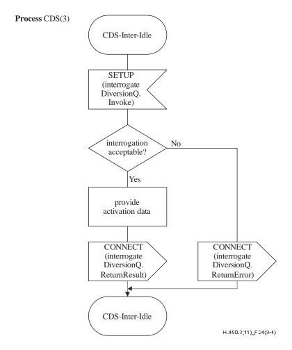
Figure 24 – CDS SDLs (sheet 3 of 4)
