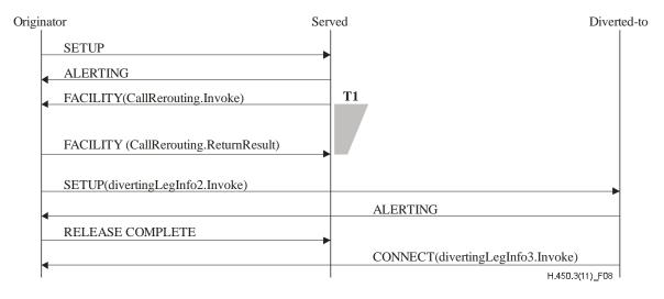
Figure 8 - Signalling flow for call forwarding delayed (CFNR, CD) with rerouting
