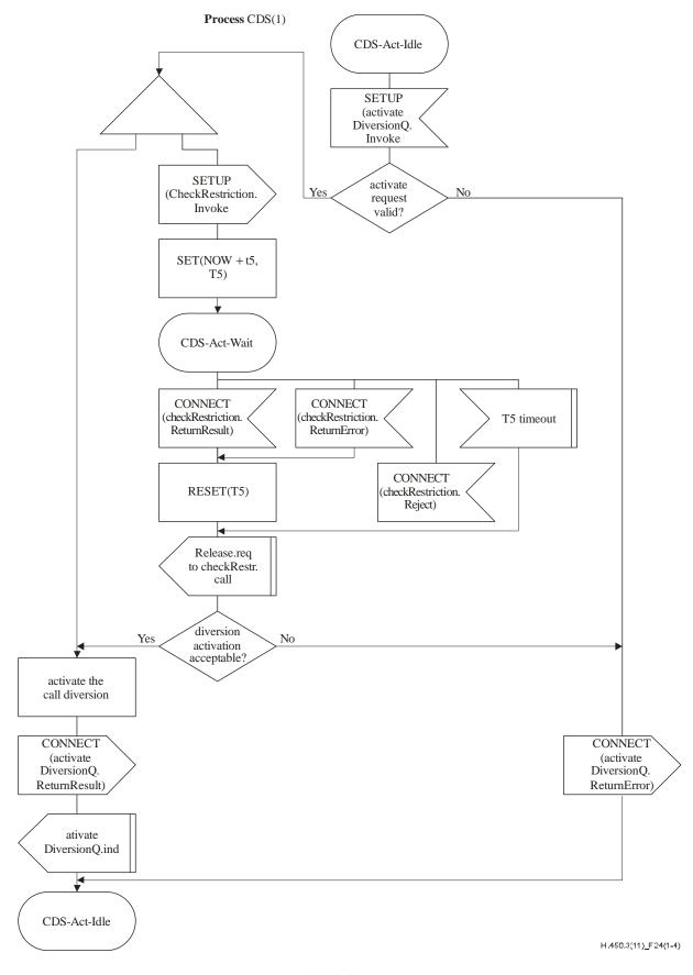
Figure 24 – CDS SDLs (sheet 1 of 4)
