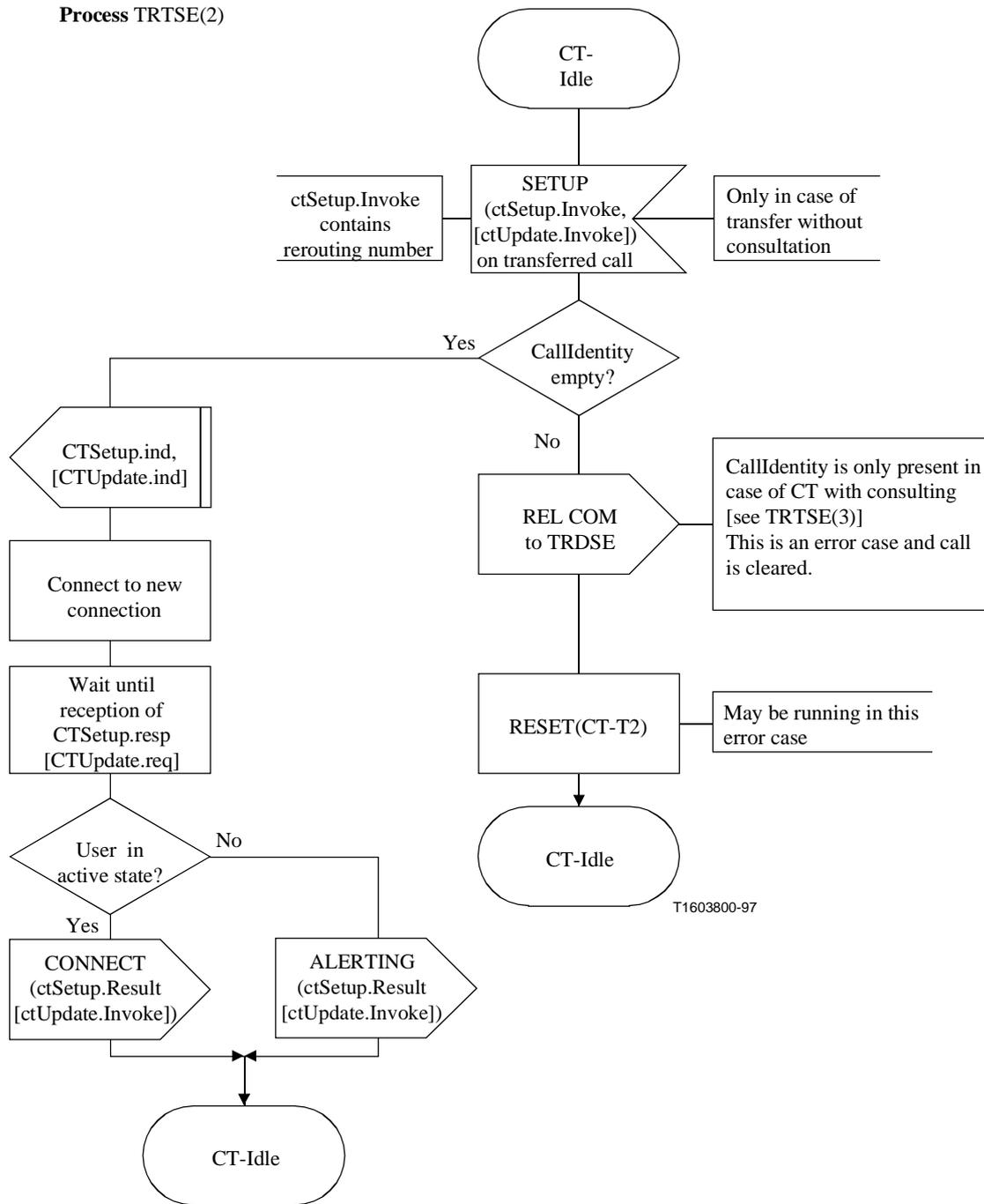
Figure 23/H.450.2 (sheet 2 of 3) – Secondary signalling entity
