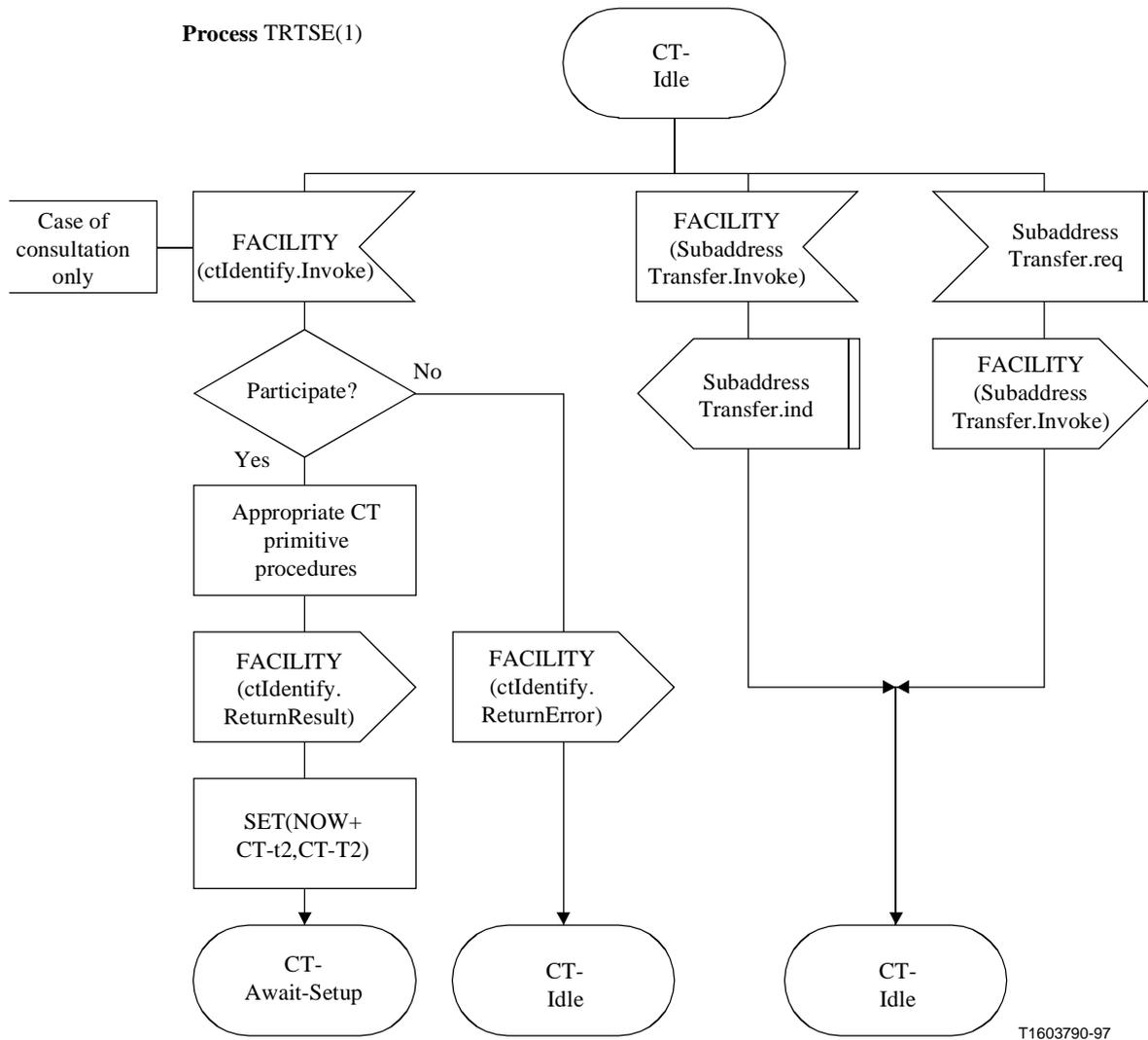
Figure 23/H.450.2 (sheet 1 of 3) – Secondary signalling entity
