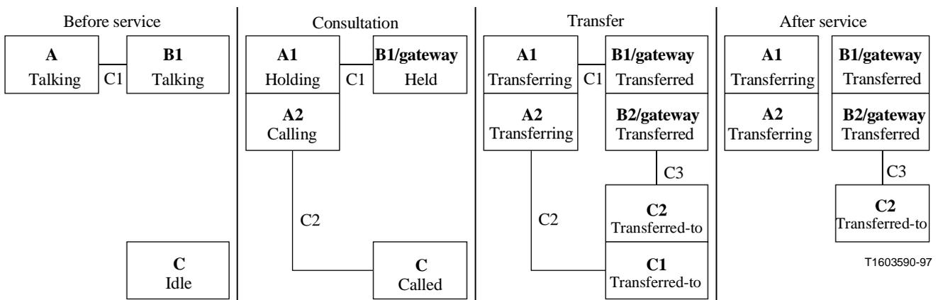
**Figure 7/H.450.2 – Operational model for transfer with secondary call**
