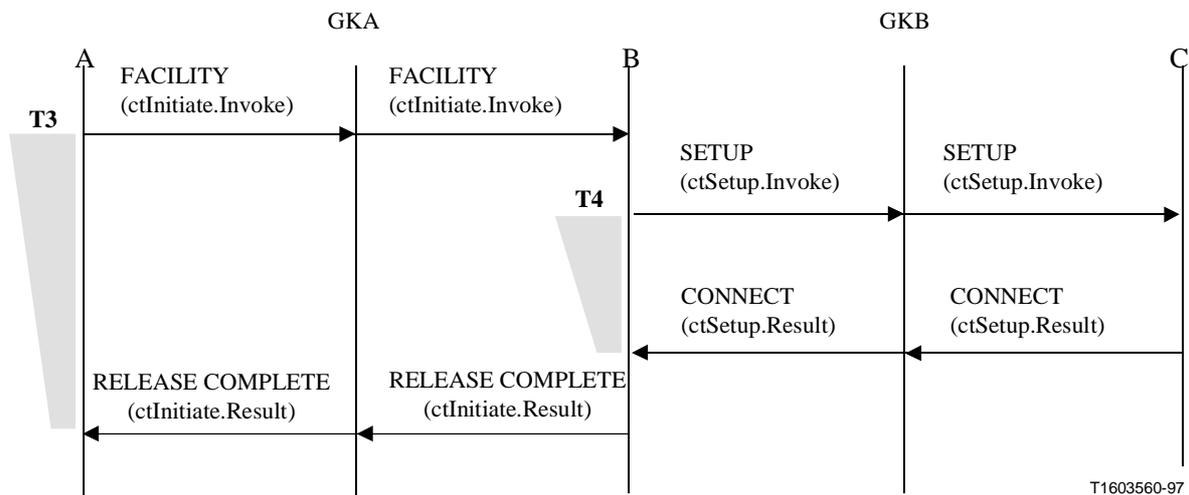
**Figure 4/H.450.2 – Signalling flow for transfer using gatekeeper routed model – GK is transparent for call transfer operations**
