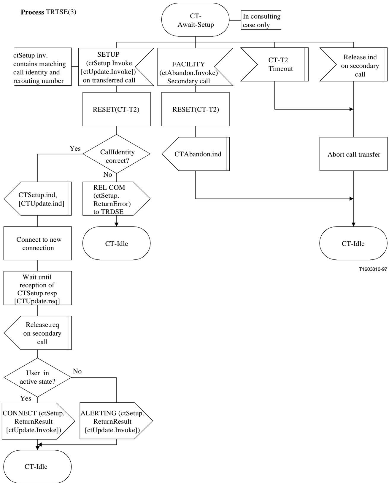
**Figure 23/H.450.2 (sheet 3 of 3) – Secondary signalling entity**
