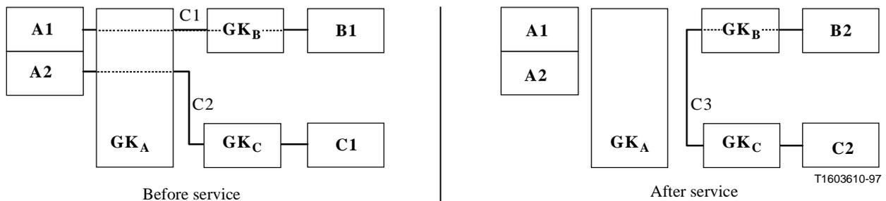
**Figure 9/H.450.2 – Operational model for call transfer with consultation – GK is transparent for call transfer operations**
