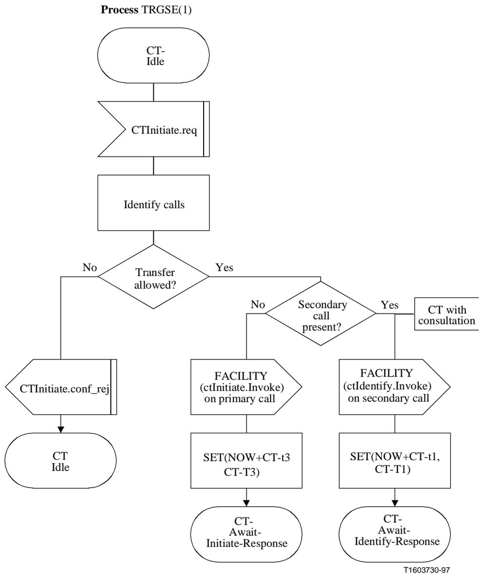
**Figure 21/H.450.2 (sheet 1 of 3) – Transferring signalling entity**
