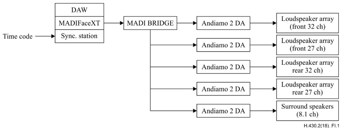
Figure I.1 – Block diagram of immersive sound reproduction system
