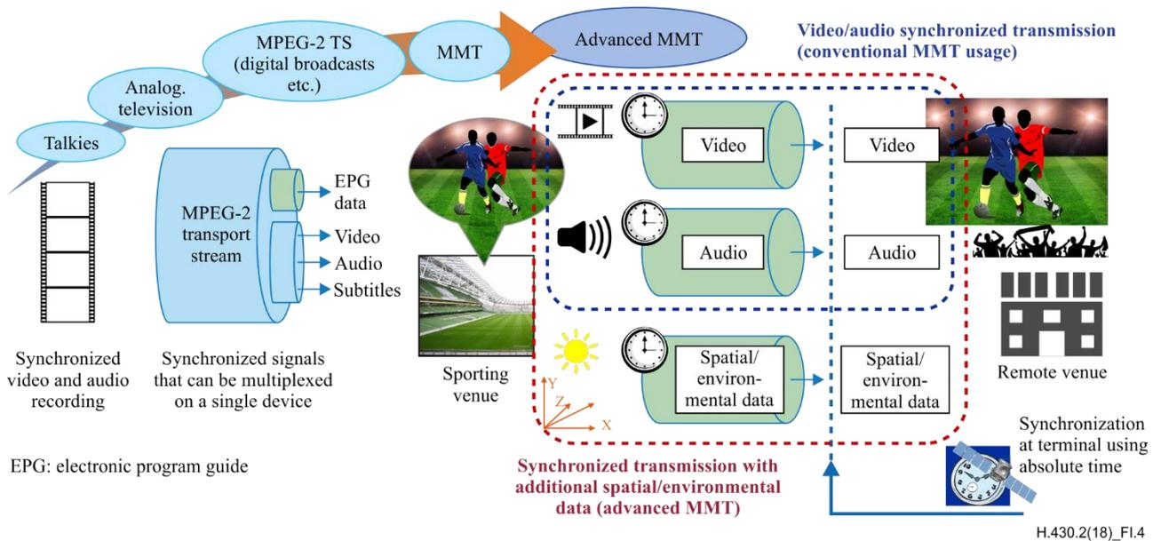
**Figure I.4 – Media synchronization for realistic sensation (Advanced MMT)**
