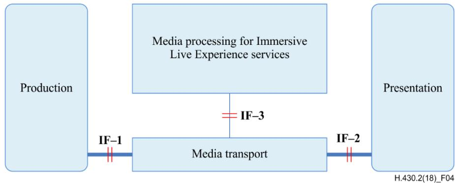
**Figure 4 – General role model for providing ILE services**
