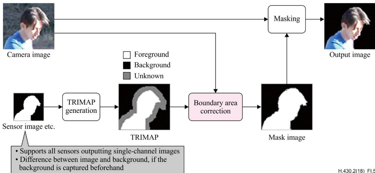
**Figure I.5 – Overview of arbitrary background object extraction process**
