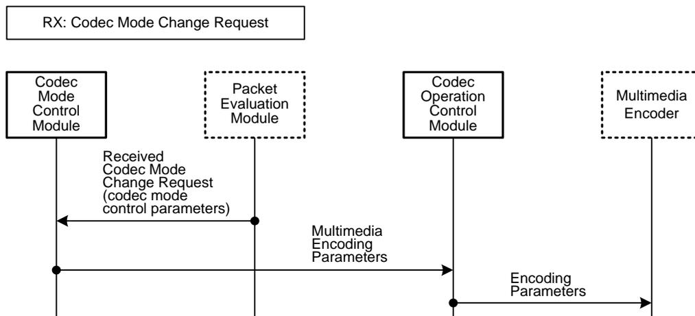
Figure 9 – Signalling flow to apply the received codec mode change request
