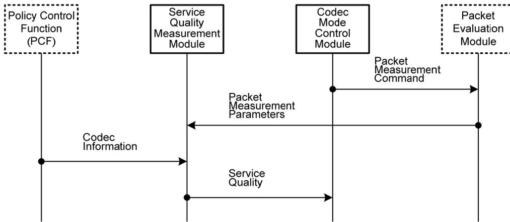
**Figure 7 – Signalling flow to measure the service quality**
