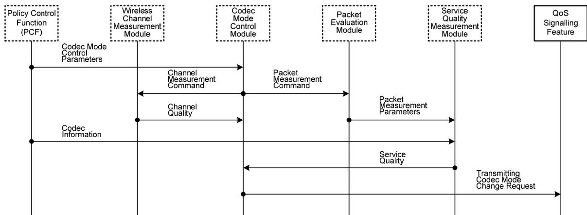
**Figure 14 – Detailed message exchange sequences for the transmitted codec mode decision procedure**
