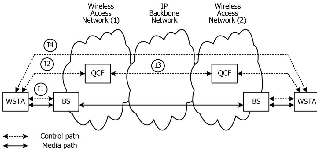
**Figure 1 – Conceptual reference network architecture for adaptive QoS control using variable bit-rate codecs**
