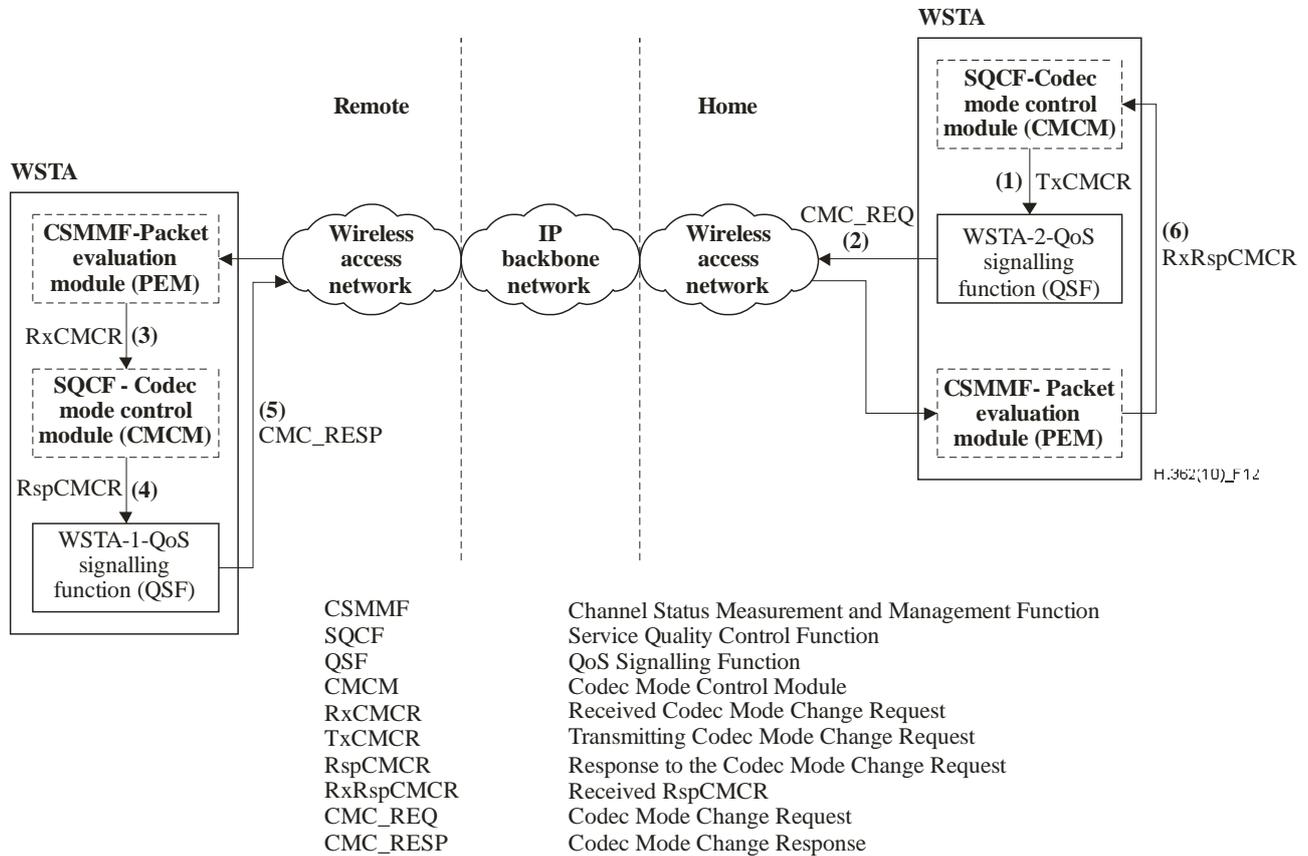
**Figure 12 – QoS signalling function (QSF)**
