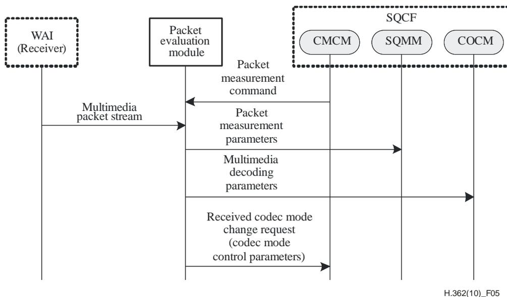
**Figure 5 – Signalling flow for the packet evaluation module (PEM)**
