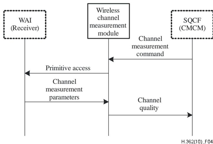
**Figure 4 – Signalling flow for the wireless channel measurement module (WCMM)**
