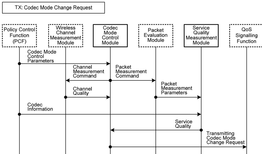
**Figure 8 – Signalling flow to change the codec mode of the remote WSTA**
