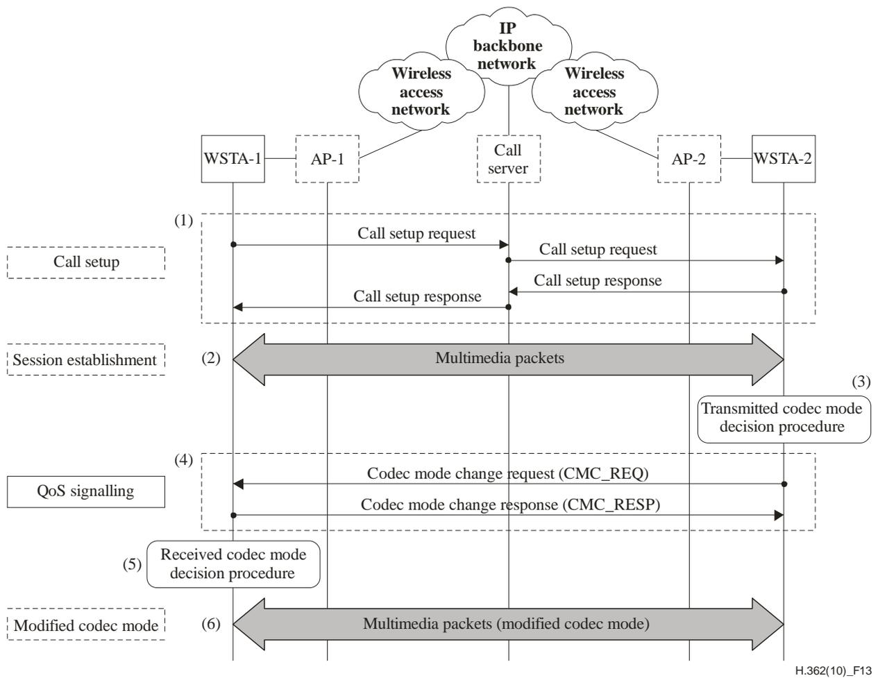
**Figure 13 – Procedure for QoS signalling message exchange**
