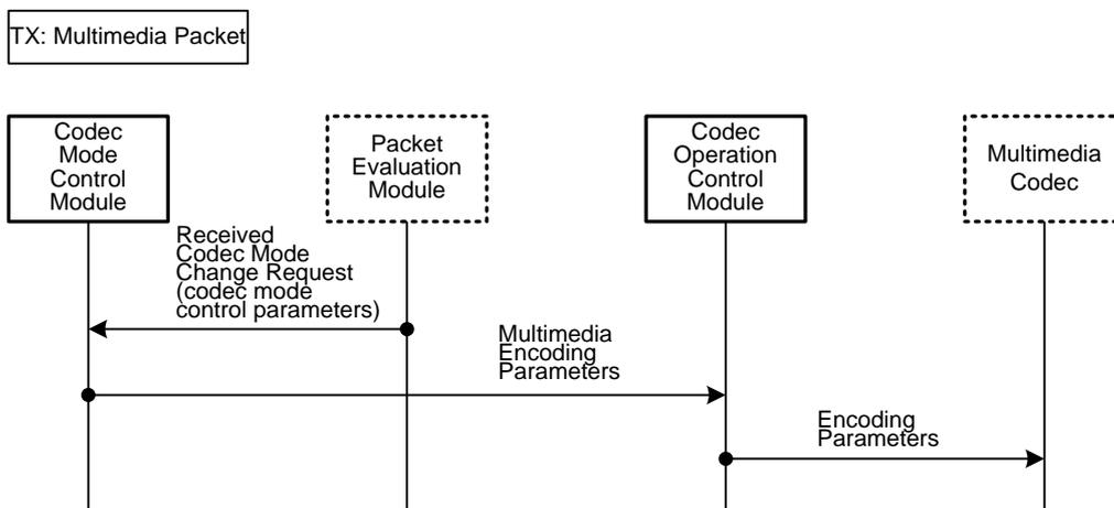
**Figure 11 – Signalling flow to apply the multimedia encoding parameters**
