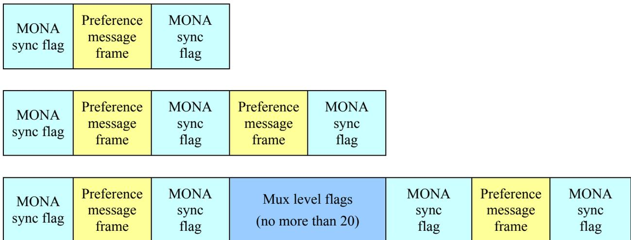
**Figure K.1/H.324 – Illustration showing several acceptable patterns of MONA sync flags, MONA preference message frames, and multiplexer level stuffing flags**
