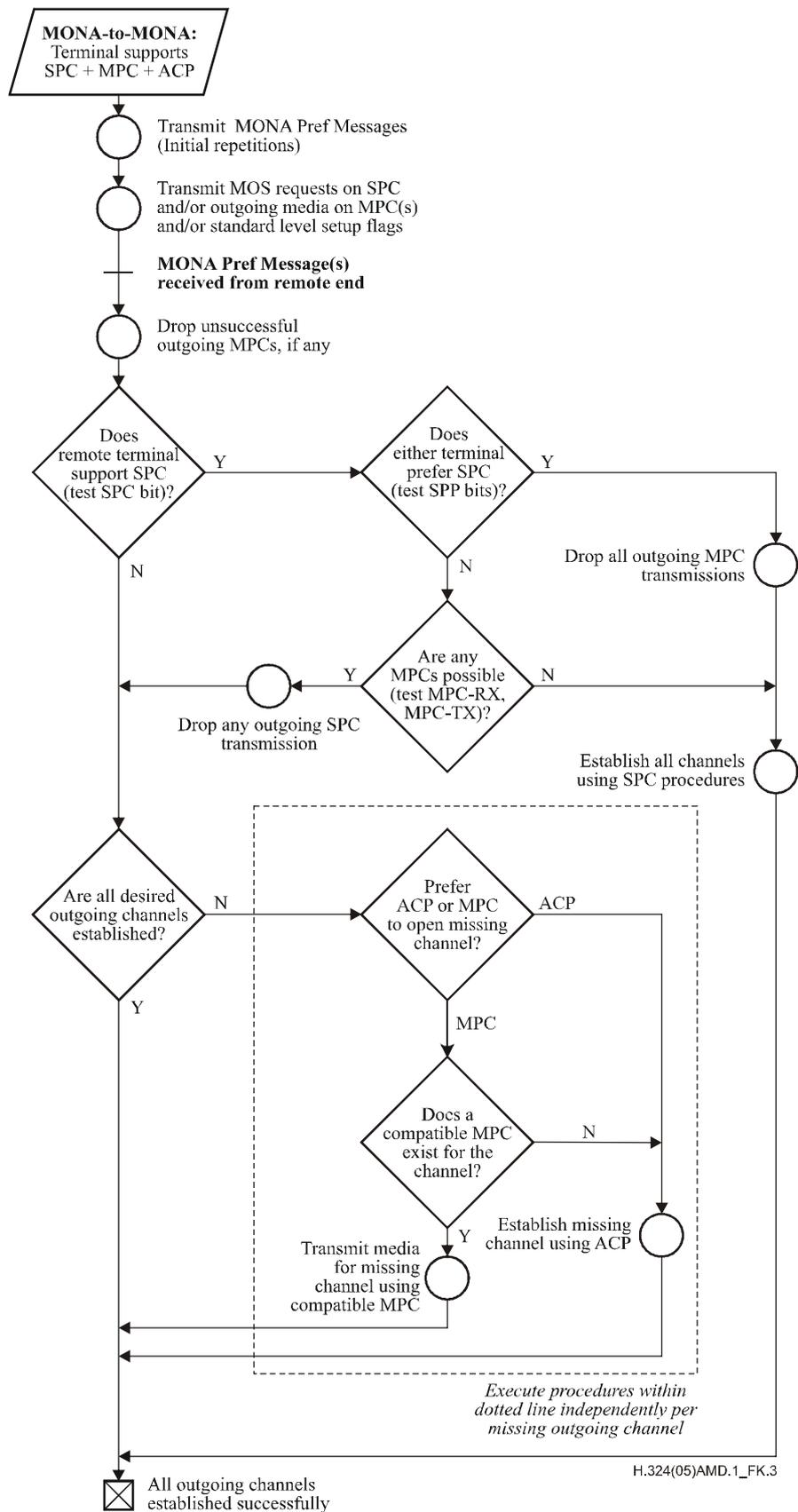
**Figure K.3/H.324 – Logic typically used by a Class I MONA terminal to establish outgoing audio and video channels to a remote MONA terminal**
