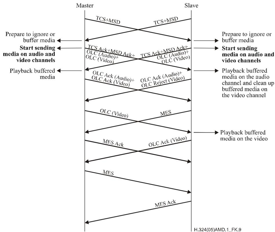
**Figure K.9/H.324 – Channel rejection during accelerated H.245 procedures**
