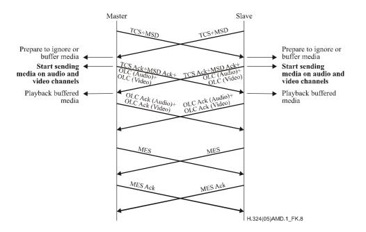
Figure K.8/H.324 – Accelerated H.245 procedures for both audio and video channels
