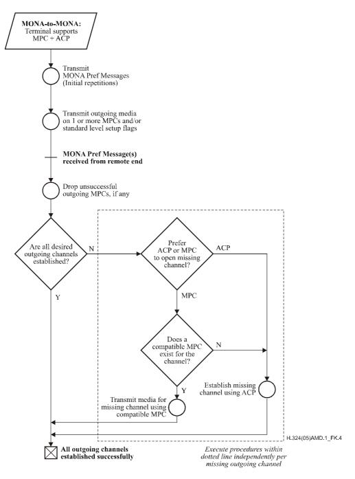
Figure K.4/H.324 – Logic typically used by a Class II MONA terminal to establish outgoing audio and video channels to a remote MONA terminal
