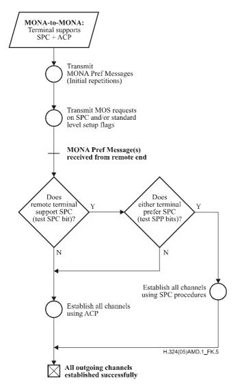
Figure K.5/H.324 – Logic typically used by a Class III MONA terminal to establish outgoing audio and video channels to a remote MONA terminal
