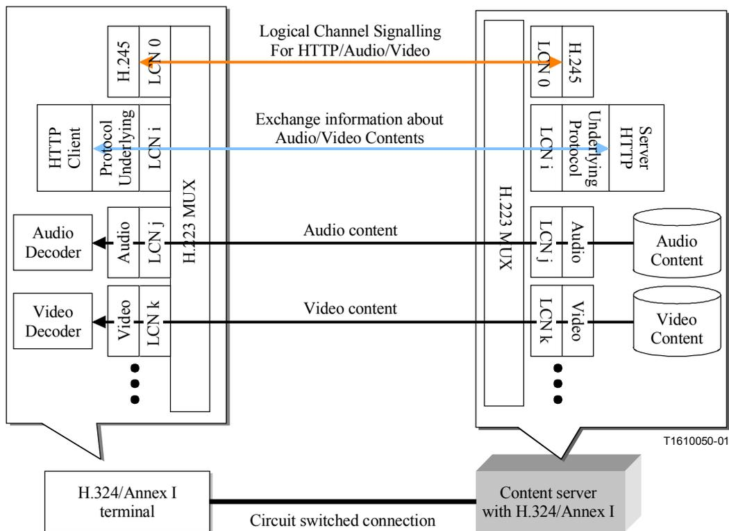
**Figure I.1/H324 – An application using H.324 Annex I**
