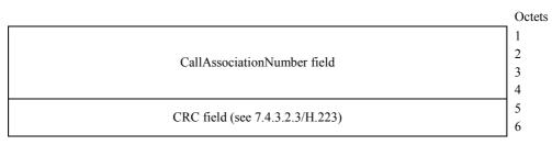
Figure 7/H.324 – Payload for *request additional* control frames
