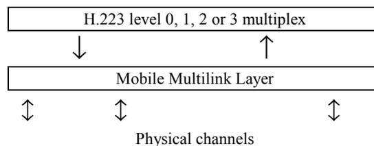
**Figure 1/H.324 – Overview of the mobile multilink layer**
