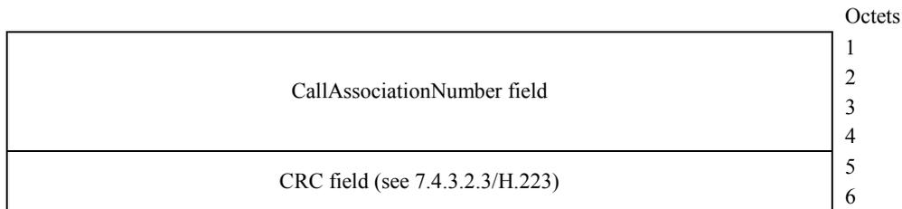
Figure 7/H.324 – Payload for *request additional* control frames
