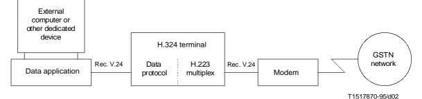
FIGURE 2/H.324 Data application – Data protocol interface
