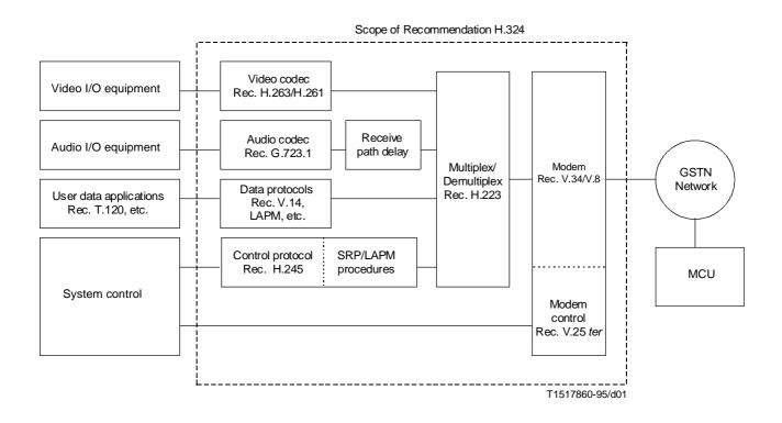
FIGURE 1/H.324 Block diagram for H.324 multimedia system
